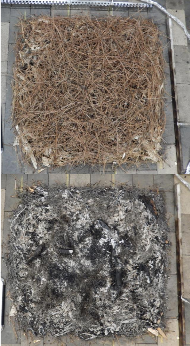
Figure 5. Before (top) and after (bottom) pictures of lab fuel bed burned. Fuel bed was laid out within a chalked 0.75 m X 0.75 m square.
