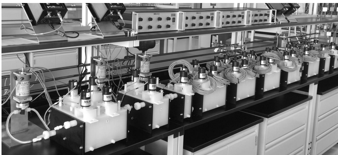
Figure 15: INL's 32 stage MEAB mixer-settler system.
