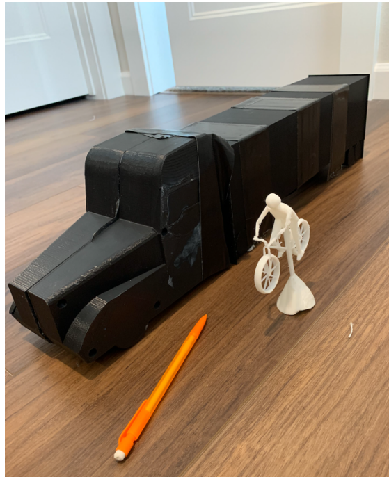
Figure 3.10 Scaled semitrailer truck and cyclist used in the wind tunnel simulations
