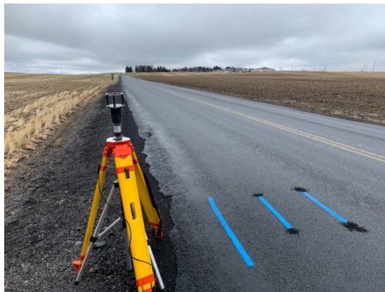
Figure 3.5 Location of marks on pavement for various side distances.
