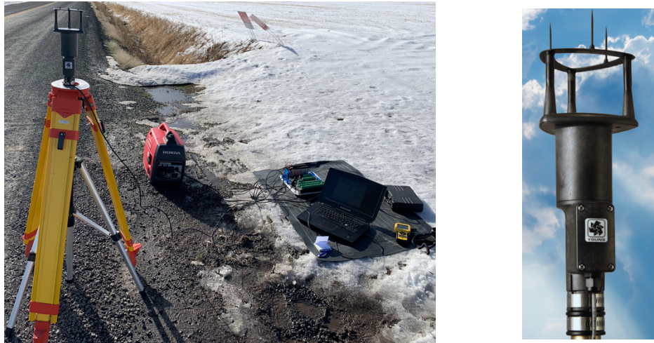
Figure 3.2 Test setup and UWS (Young 86000 anemometer).
