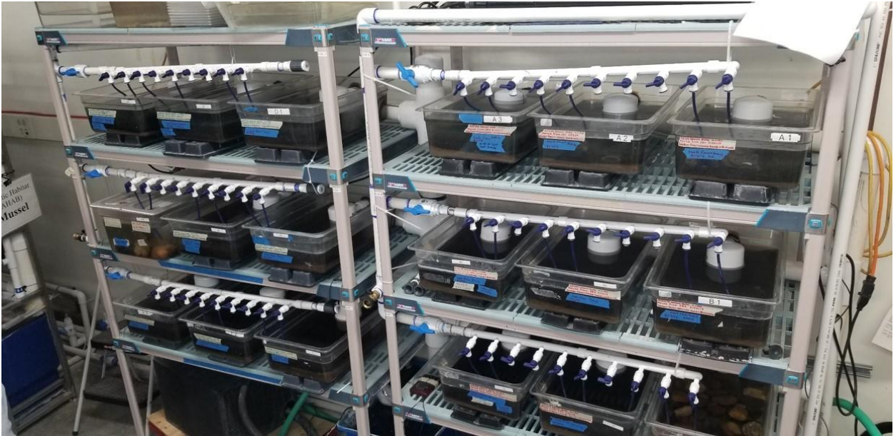
Figure 4-1. The two identical recirculating systems that were used for polyculture (left) and monoculture (right) rearing of larval lamprey. Eight tanks on each system were used to house larval lamprey, and one tank on each system was used to house Speckled Dace (polyculture) or as a feeding control tank (monoculture). Photograph by the author.
