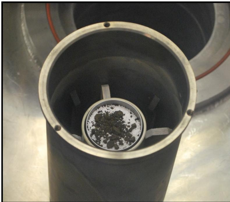
Figure 4.6: Prepared crucible for experiments with  $\text{LiCl-KCl-UCl}_3\text{-CeCl}_3$ .
