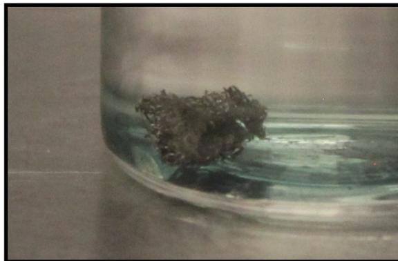
Figure 7.7: Dendrite mass produced at 450 mV condition during washing in DI water.
