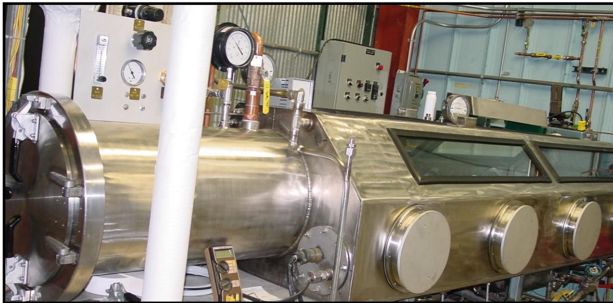
Figure 4.1: Argon-atmosphere glovebox for performance of LiCl-KCl-CeCl<sub>3</sub> experiments.
