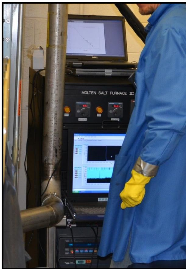
Figure 4.14: Experiment control cabinet with laptop for Corware (top), furnace power and temperature monitoring (center), and Solartron 1287 potentiostat (bottom).
