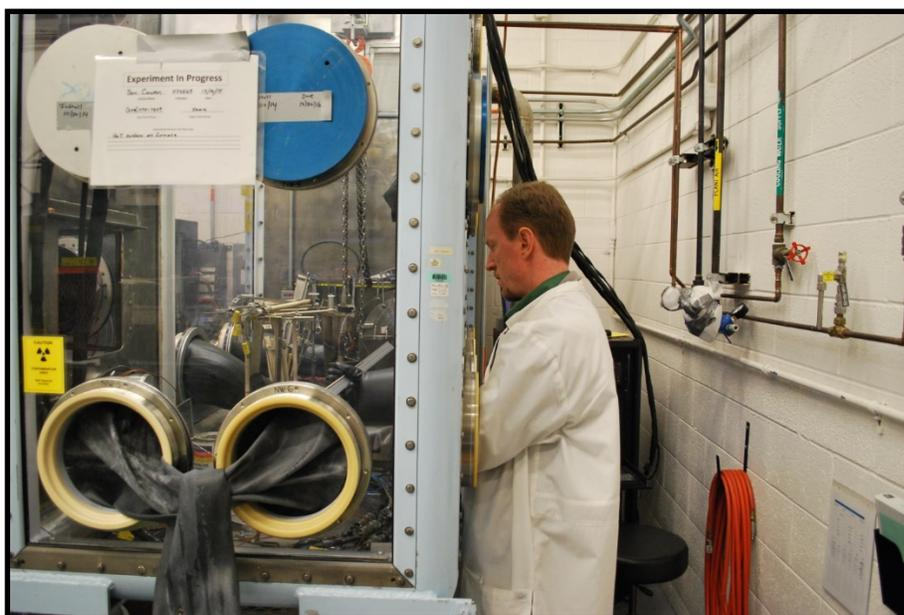
Figure 4.7: Measuring electrode length in the radiological glovebox for experiments with  $\text{LiCl-KCl-UCl}_3\text{-CeCl}_3$ .
