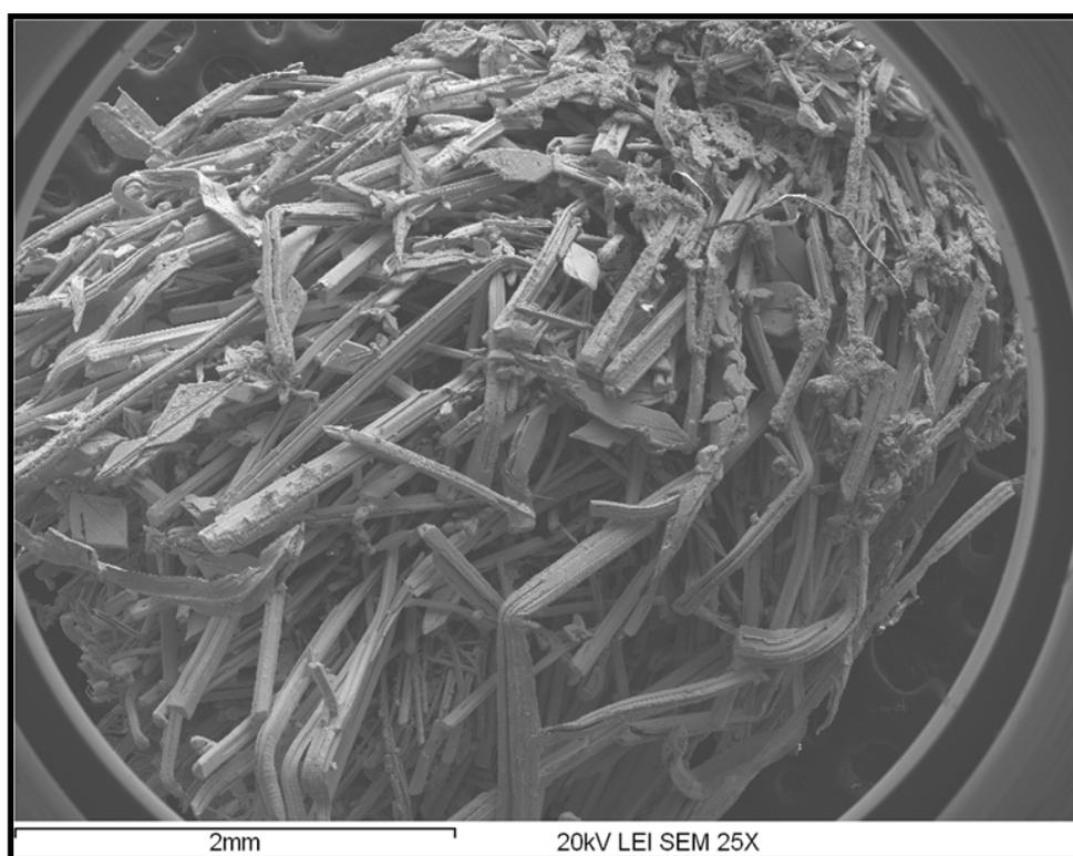
Figure 7.8: Overview of dendrite mass on SEM mount, produced at 450 mV condition.
