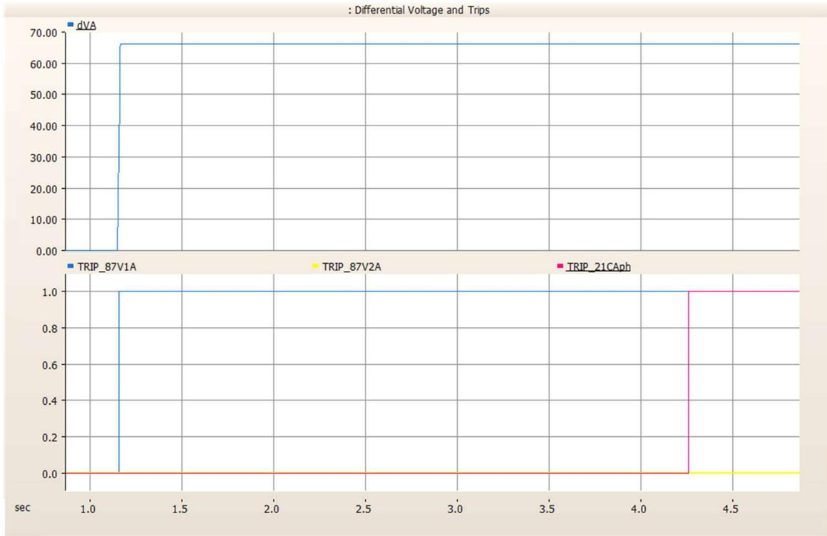
Figure 7.9: Differential voltage and trip signal versus time illustrating a LVC failure with additional bank element failures
