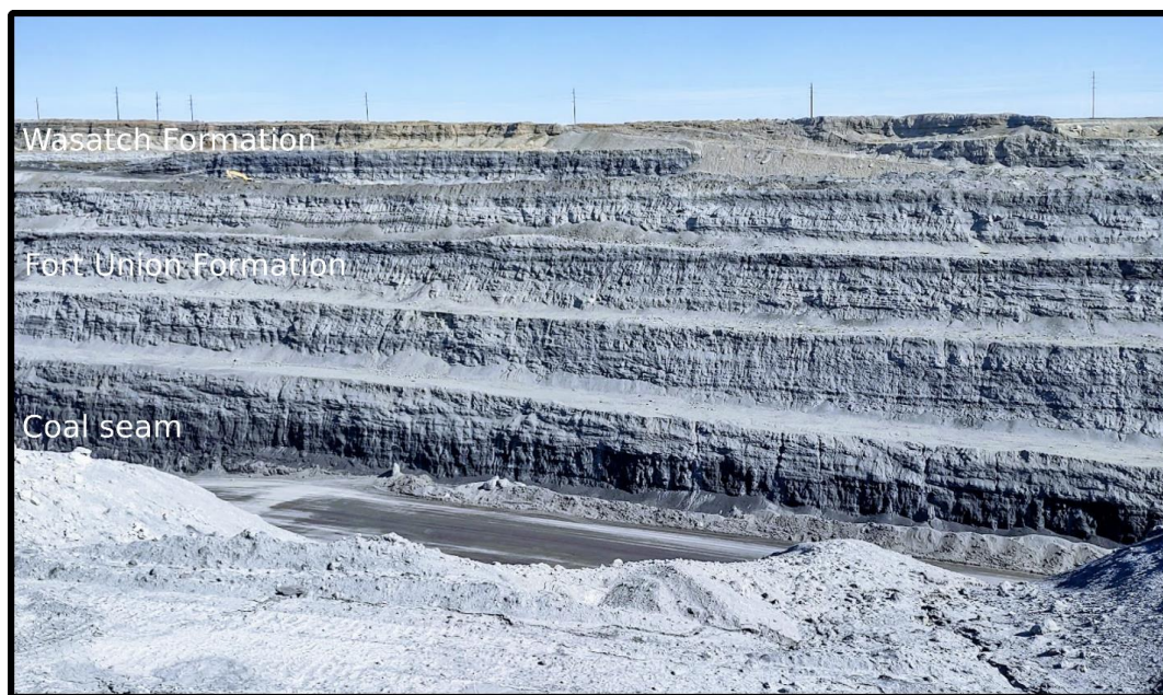
Figure 2.1 Overburden and coal seam at the Cordero Rojo Mine, Powder River Basin, Wyoming, USA.
