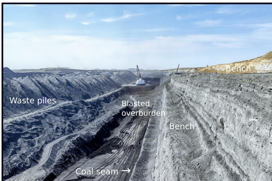
Figure 2.2 Removal of overburden and waste rock generation during open-pit coal mining at the Cordero Rojo Mine, Powder River Basin, Wyoming, USA.
