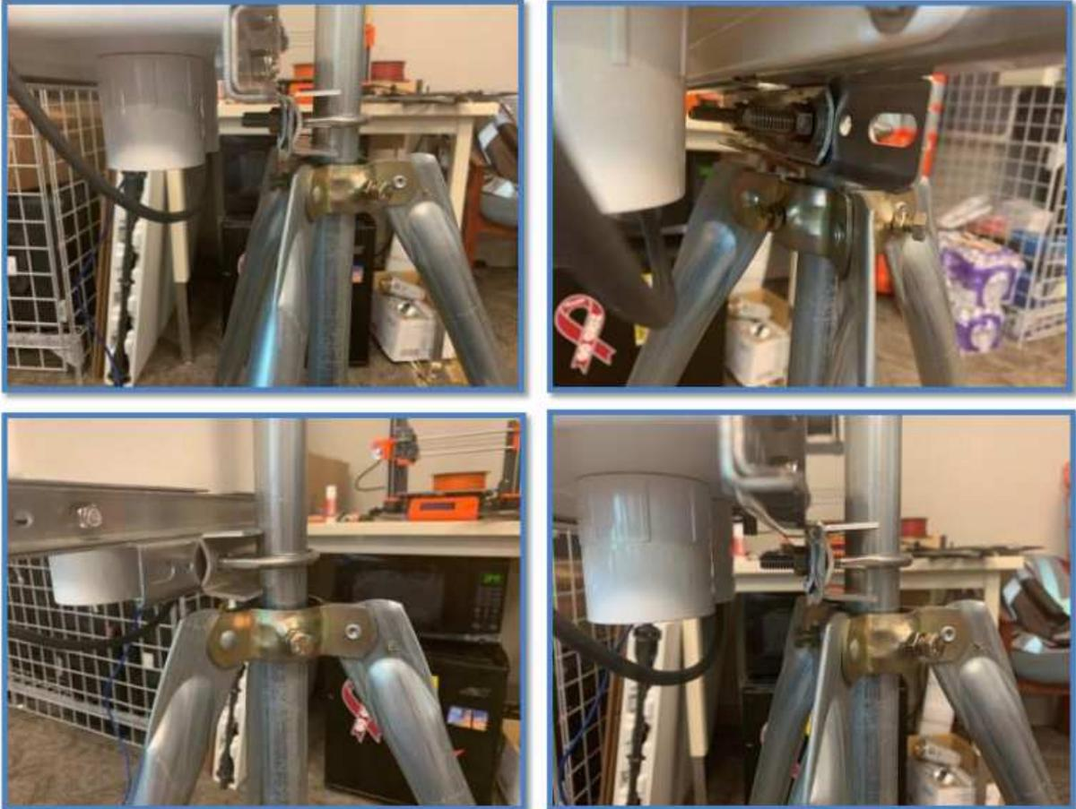
Slide the metal rod with the Lufft sensor on the end (with the stopper firmly attached) and datalogger box attached, into the opening in the stand.
