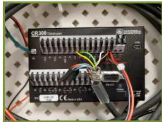
Hook the solar panel to the Lufft datalogger by putting the leads through the unused hole in the bottom of the datalogger box and into the CHG +/- port on the right-hand side of the CR300 datalogger (see pictures below; red is positive and black is negative).
