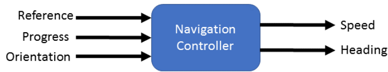
Figure 3.6: Block diagram with variables that are needed control the motors on the robot
