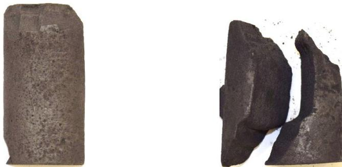
Figure 5.2: Failures typical of untrimmed (left) and trimmed (right) samples.
