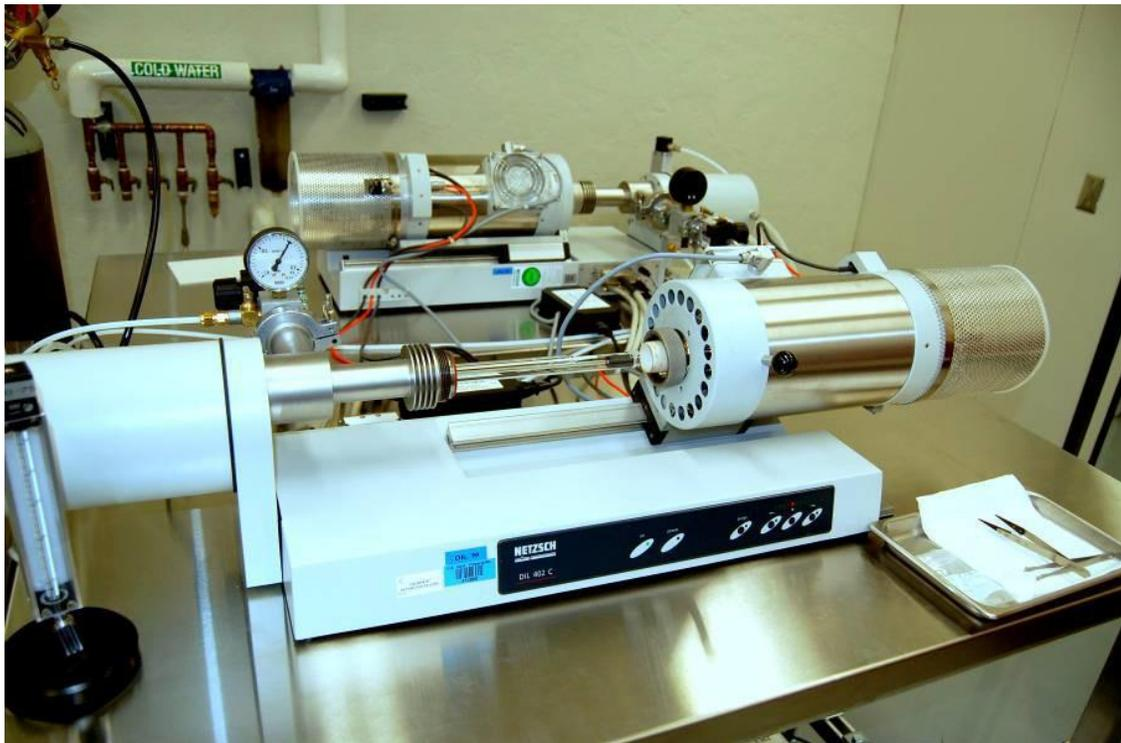
Figure 3.13: Commercial push rod Dilatometer for CTE measurement.
