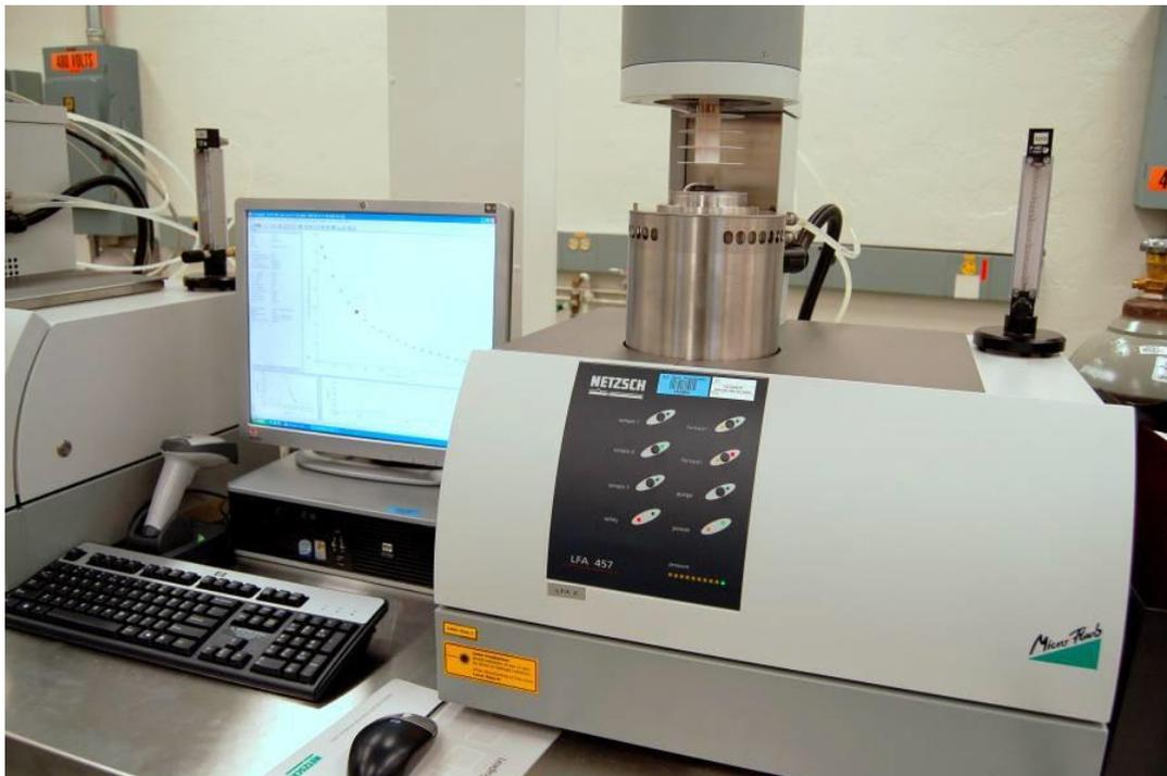
Figure 3.15: LFA measurement station for determination of thermal diffusivity.
