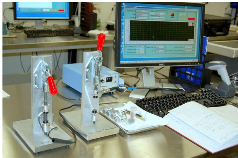
Figure 3.11: Sonic velocity measurement station.
