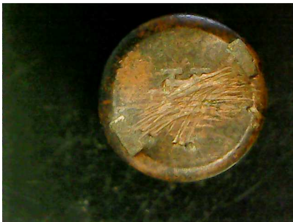
Figure 5.7. .22 caliber cartridge, fired from a Sub-Caliber adapter for a 1903 Springfield Gallery Rifle. Note the scratch marks at the center.
