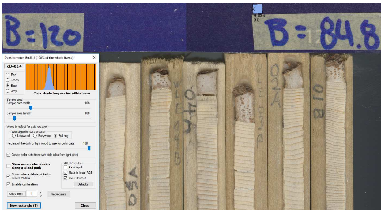
Figure 3.6: Screenshot from Coorecorder displaying blue color patches and densitometer function used for calibration.
