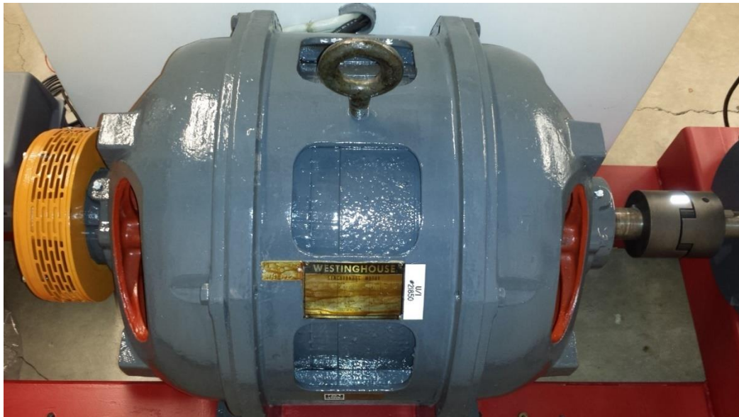
Figure 22: Lab 20 horsepower Synchronous Generator
