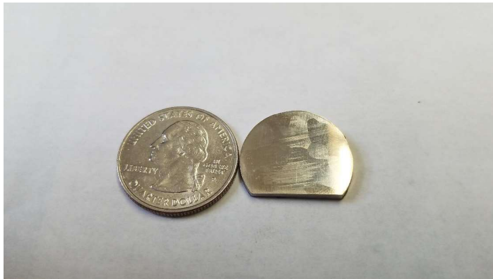
Figure 3.3.1. Zone refined nickel with visible gran boundaries next to a US quarter for size comparison.
