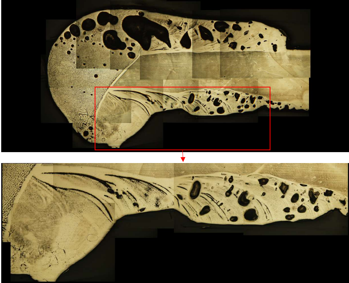
Figure 5.3.1. Magnified image of weld A on the first UI-GTAAM specimen. No grain boundaries are visible along the right side of the weld (initial start) until the deposited material beaded up (left side).
