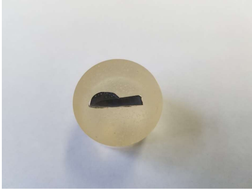
Figure 4.2.2. Image of sectioned weld cold mounted in epoxy and polished to 1 micron on a wet platen.
