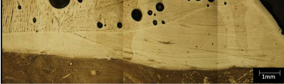
Figure 5.2.2: Enlarged optical microscopy of Region III on the bead deposited on zone refined nickel substrate.
