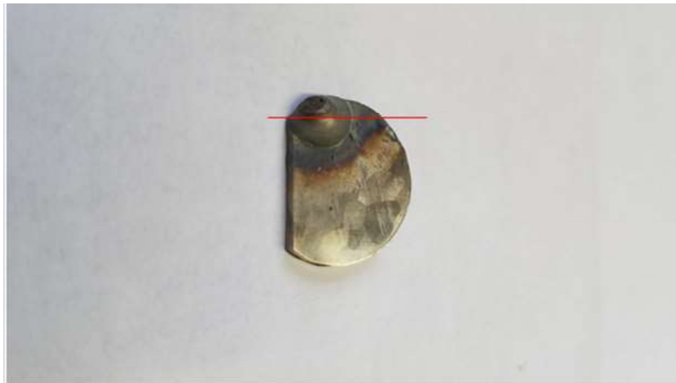
Figure 4.2.1. Zone refined nickel substrate specimen immediately following deposition of spot weld for one second. The red line illustrates the section line of the diamond saw.
