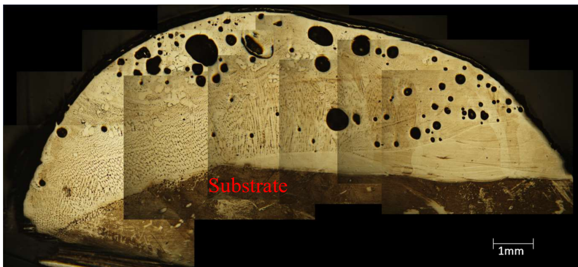
Figure 4.2.3. Optical microscopy images taken of WAAM spot weld section on zone-refined nickel specimen after applied etchant.
