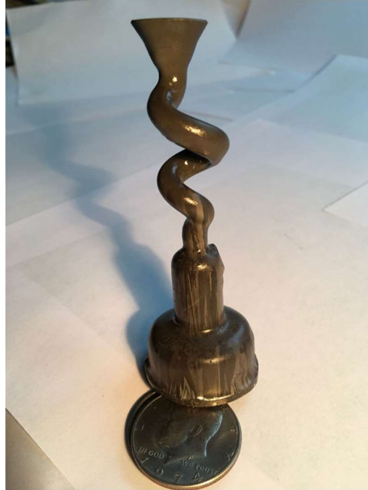
Figure 1.2.2: Helical grain selector (pigtail) of directional solidification process. Bottom of the selector starts with diverse grain orientation, towards the top grain competition results in a single grain for casting to grow on [2].
