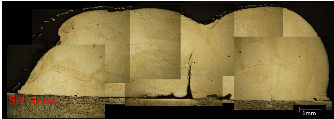
Figure 4.2.4. Optical microscopy results of Vandalforge depositions on single crystal substrate.
