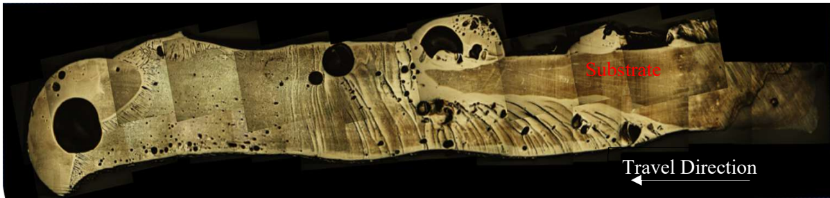
Figure 4.2.7. Cross section of continuous deposit E.
