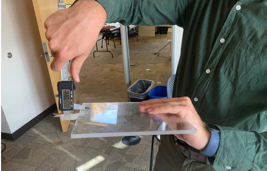
Figure 43. Image showing thickness measurement.
