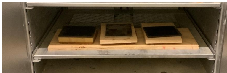
Figure 22. Guarded hot plate oven drying setup.
