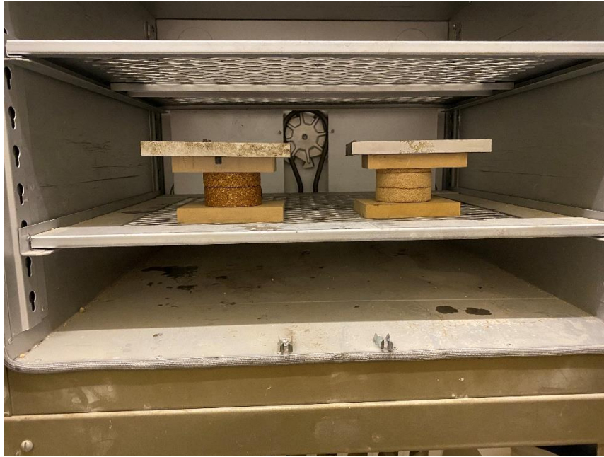
Figure 5. Needle probe oven drying setup.
