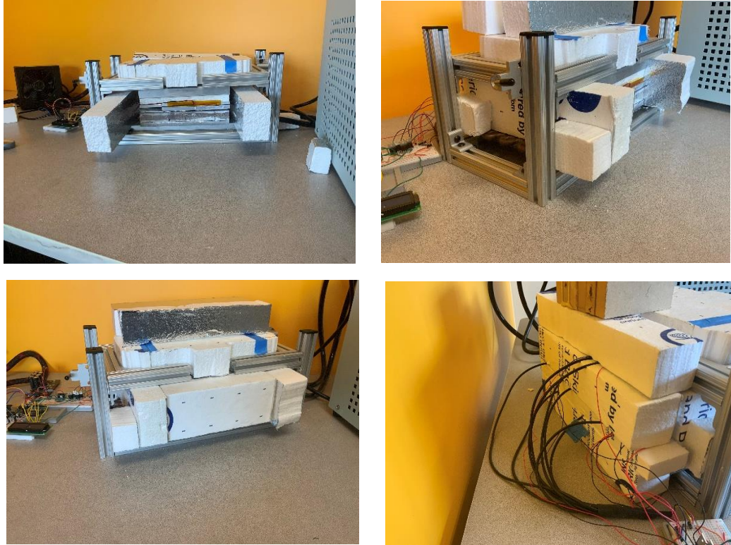
Figure 44. Process to install insulation onto the sides (top left and right), front (bottom right) and back (bottom right), of the apparatus.
