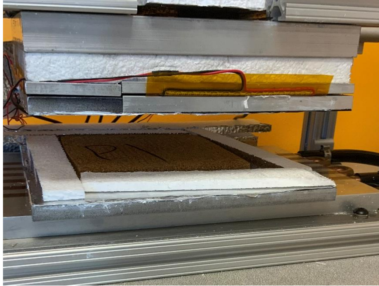
Figure 23. Insulation surrounding the sample to limit heat loss.
