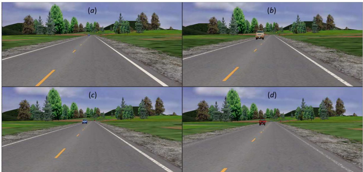
Figure 7.4: Driver simulation graphic of edgeline deterioration percentages (only 6 inch shown): (a) 0%, (b) 25%, (c) 50%, and (d) 75%
