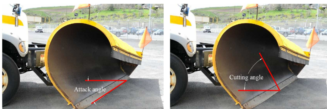
Figure 3.8: Description of the attack and cutting angles
