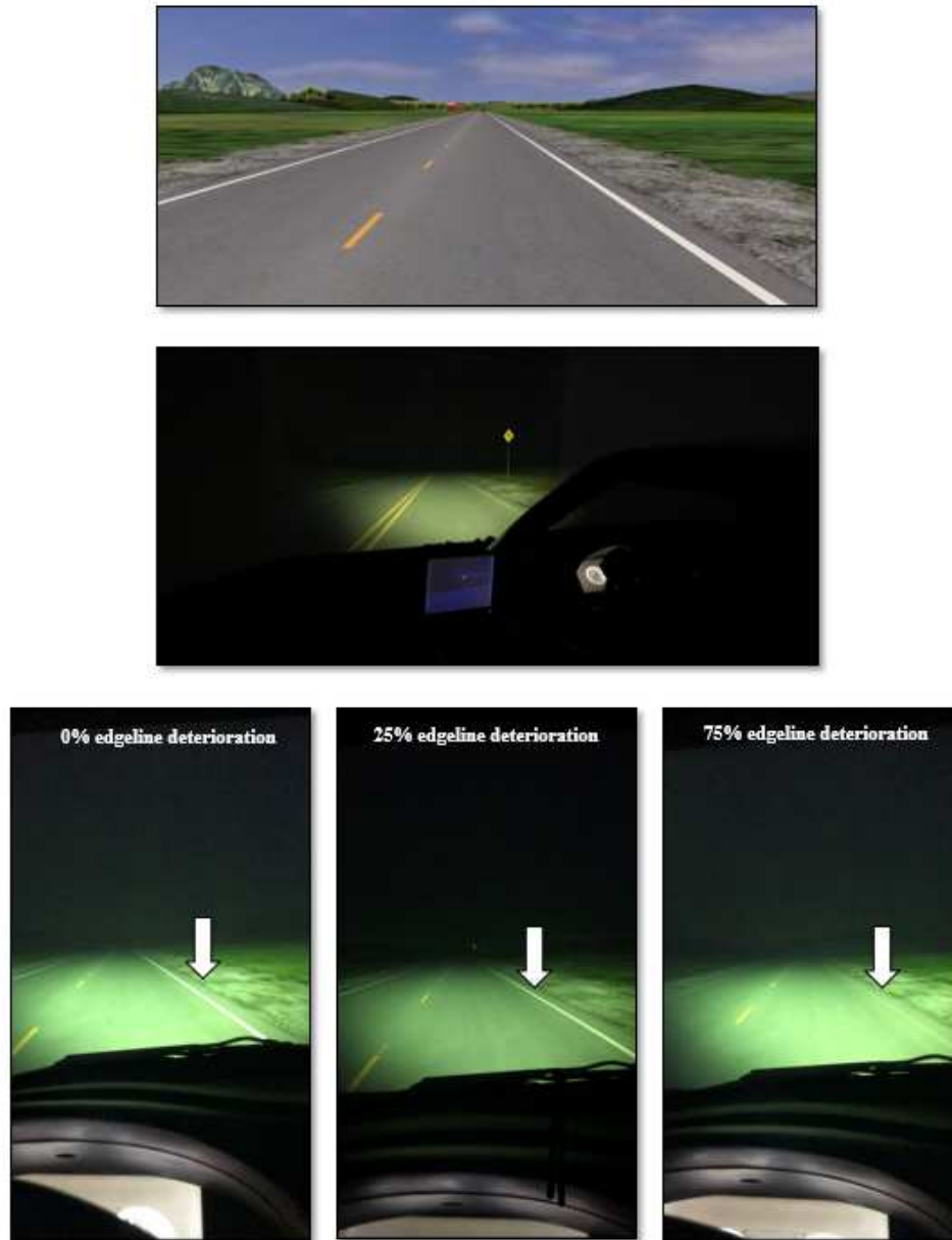
Figure 7.2: Driver simulation scene during daytime, and pictures of different edgeline deterioration levels at nighttime simulation
