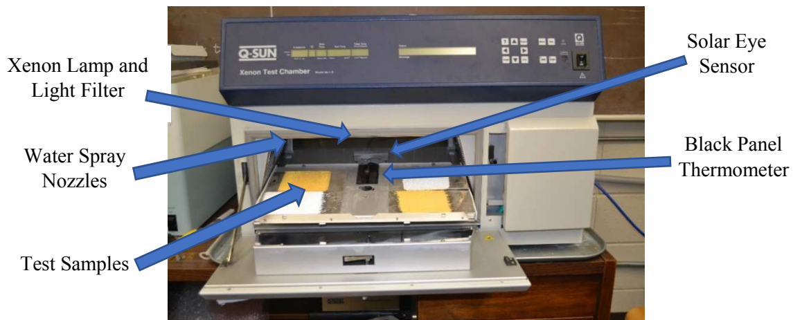
Figure 3.13: XAC components and sample configuration
