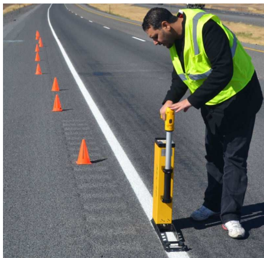
Figure 5.2: Measuring retroreflectivity at field test sites using MX 30 retroreflectometer
