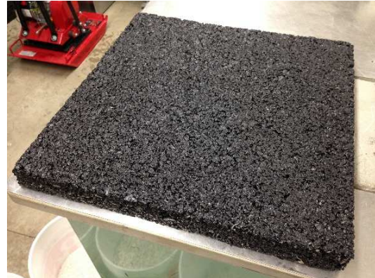
Asphalt slab after compaction
