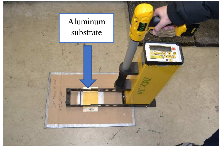
Figure 3.18: Retroreflectivity measurement on aluminum substrate
