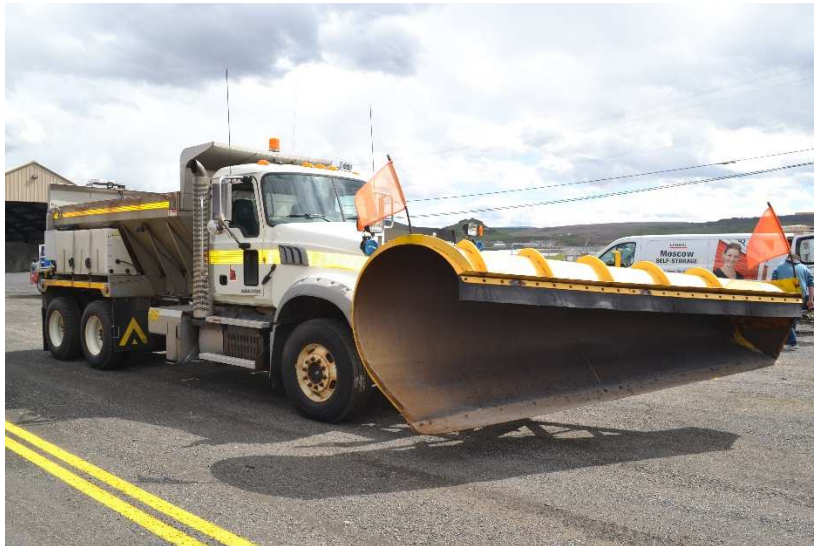
Figure 3.7: Front-mounted plow on tandem dump truck used in Idaho
