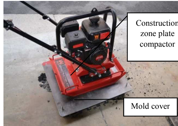
Construction zone plate compactor
