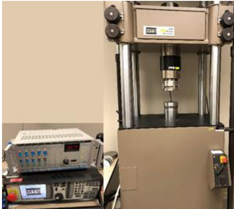
Fig. 3.5: Material testing machine (MTS) used for Quasi-static tests.
