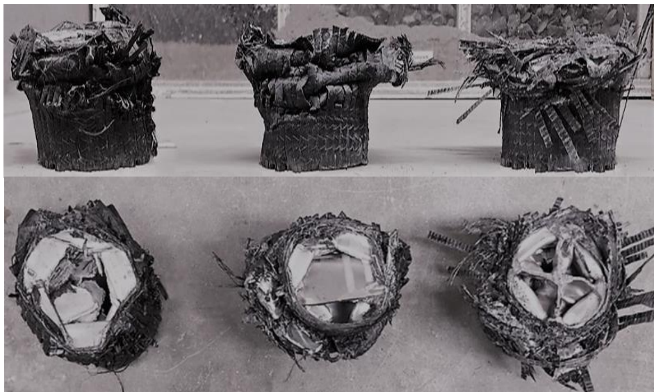
Fig. 3.7: Hybrid specimens after axial crushing.
