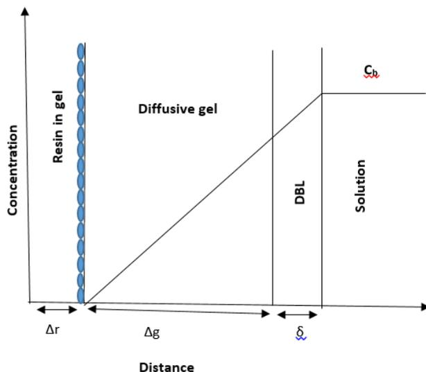
**Figure 3.1** Schematic representation of the free concentration of ionic species in a hydrogel assembly in contact with the aqueous solution, where the concentration is  $C_b$  (DBL is diffusive boundary layer). The rate of diffusion is assumed to be the same in the gel and solution. (Zhang and Davison, 1995)
