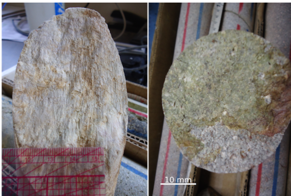
Figure 2.3: Alteration on fracture surfaces of welded tuff core. Left) Potential slickenlines on core located near inferred fault. Right) Common alteration seen forming a skin on fracture surfaces.
