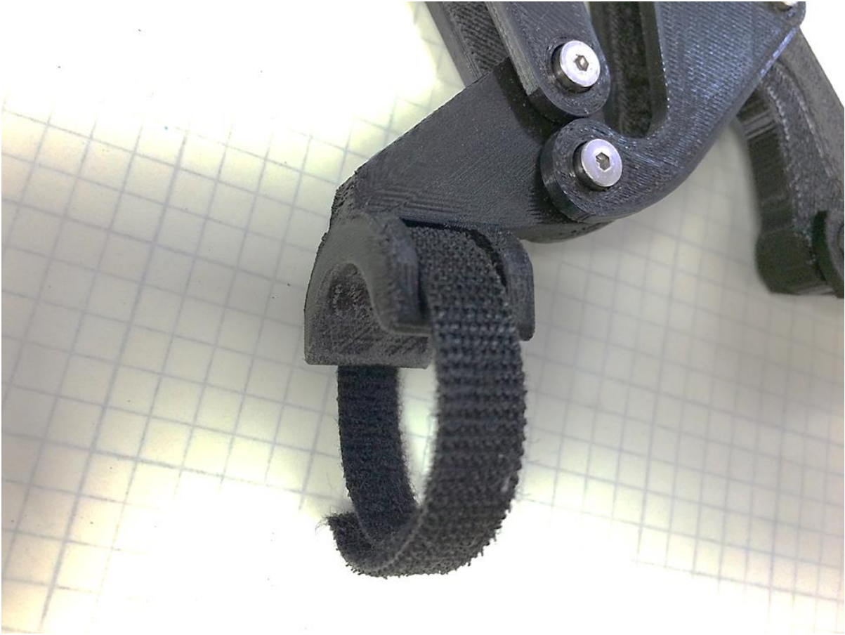
Figure 25. Close-up of interface between thumb and mechanism featuring a hook and loop strap.
