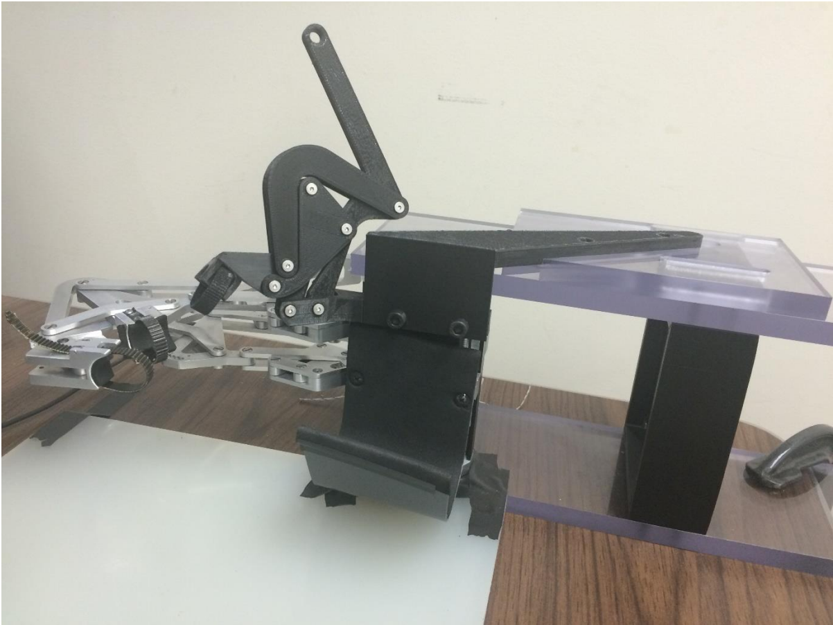
Figure 22. Full rapid prototyped mechanism with exoskeleton and adjustable base shown attached to a mockup of the housing for FINGER.
