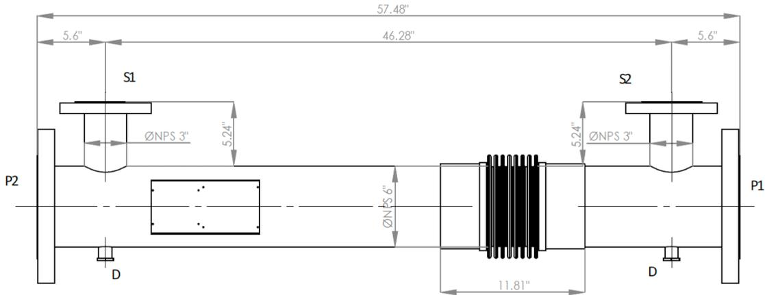
Figure 2-13. Side View of HX-01 With Dimensions
