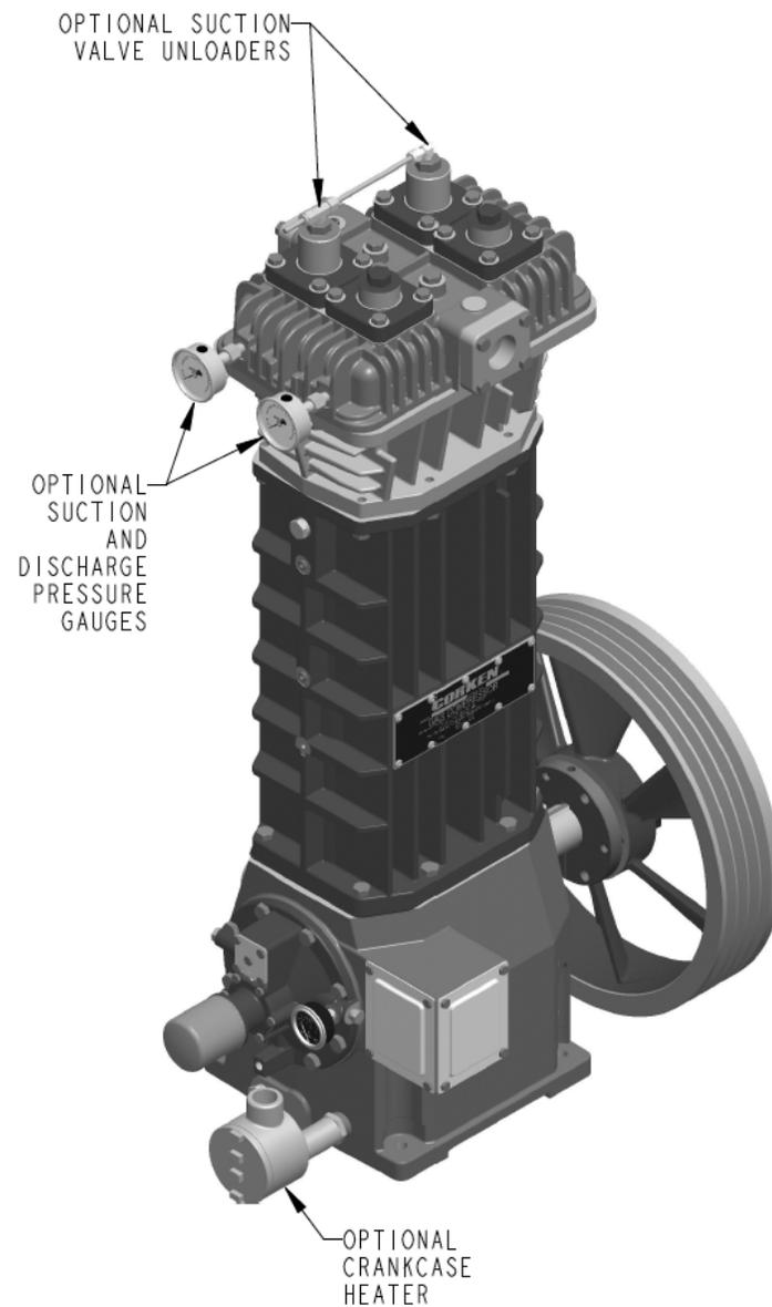
Figure 2-5. Rendering of CAD Model of Corken Compressor from Product Installation and Operation Manual
