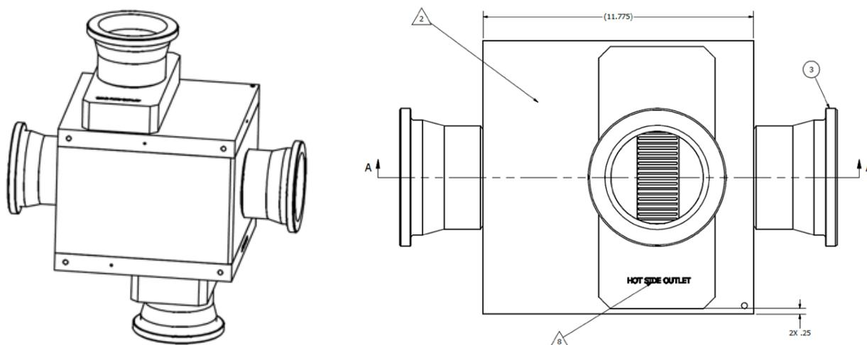
Figure 2-7. Isometric and Plan Views of HEXCES CPHX
