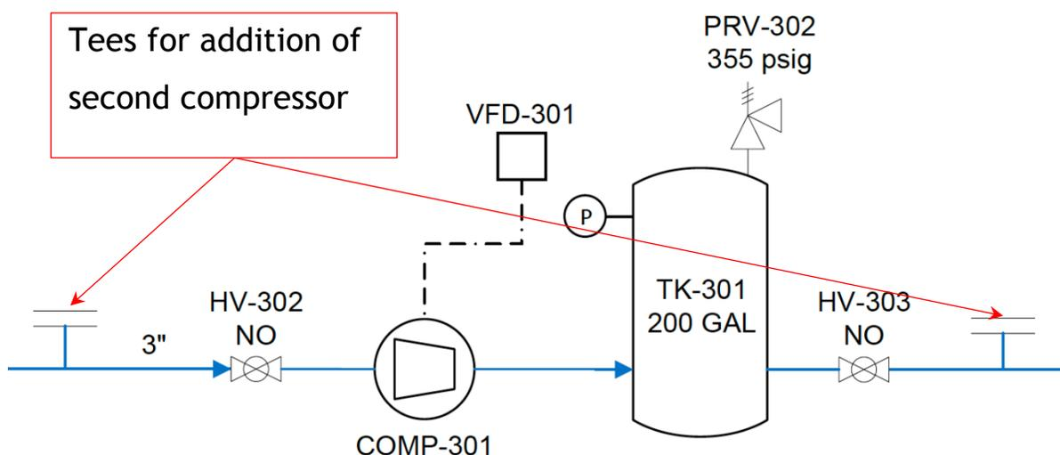
Figure 2-6. Section of P&ID Denoting Location of Tees for Additional Compressor
