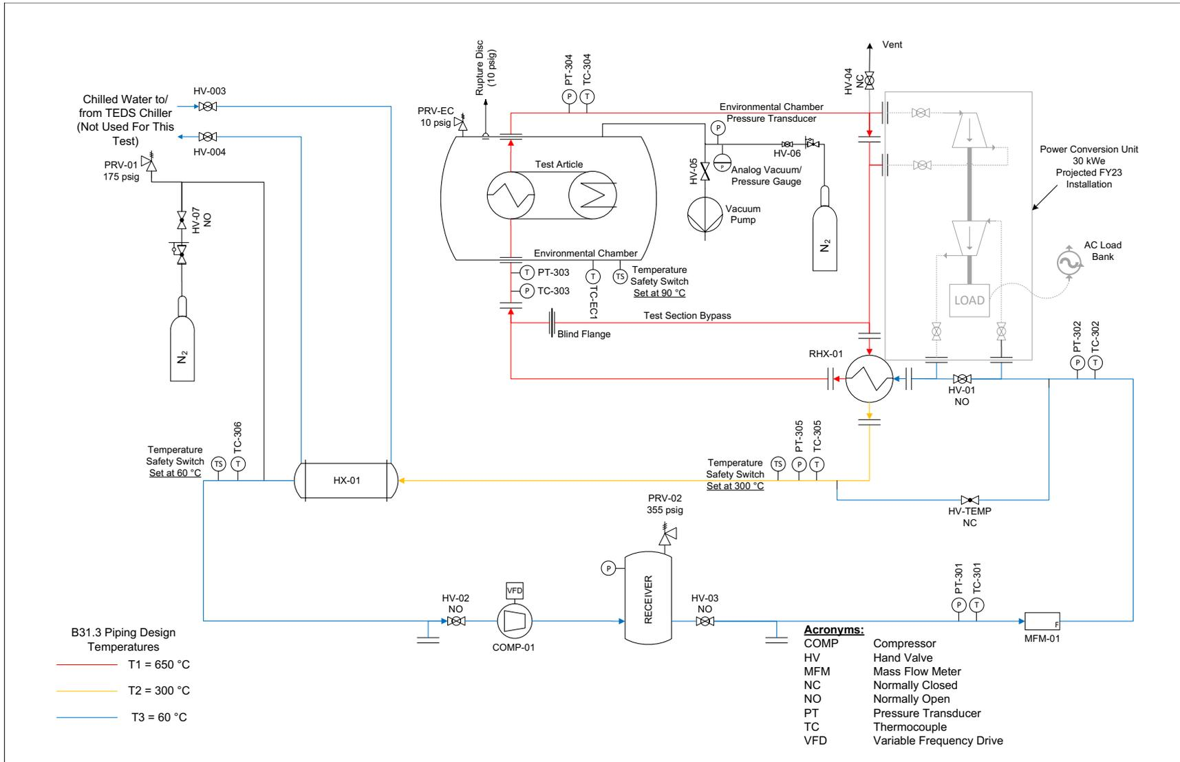
Figure 2-1. MAGNET Process and Instrumentation Diagram (P&ID)
