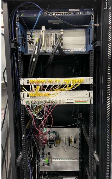
Figure 2-15. Data Acquisition Cabinet with Computer, Input/Output Cards, and Power Supplies
