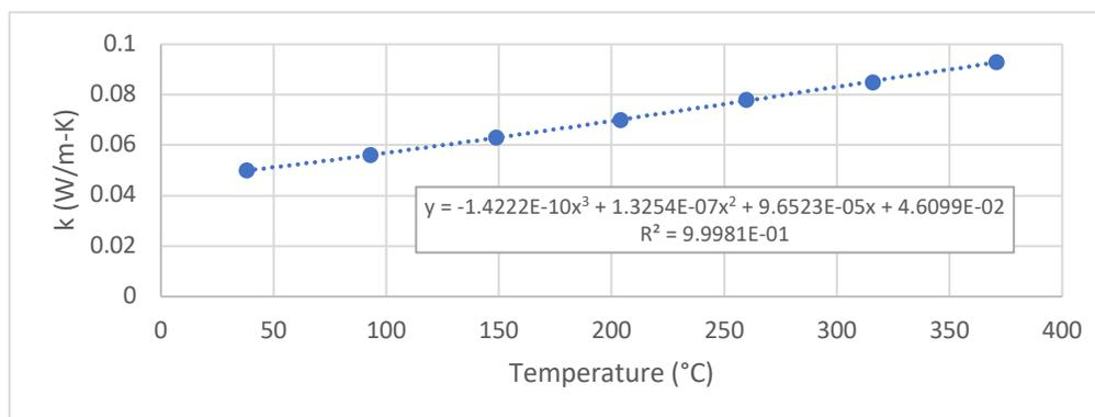
Figure 3-1. Curve Fit of Insulation Properties
