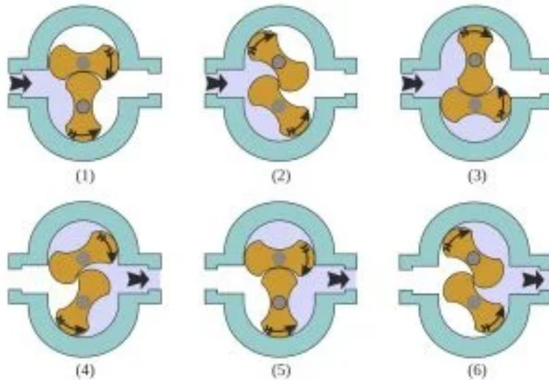
Figure 2-2. Two-Lobed, Roots-Type Blower General Operating Principal Diagram (Roots Systems, Ltd., 2023)
