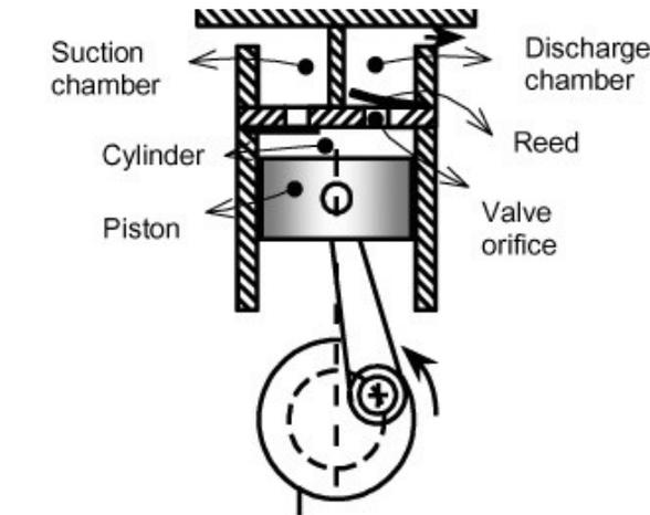
Figure 2-4. Diagram of a Single Cylinder Reciprocating Compressor (Liquip, 2023)
