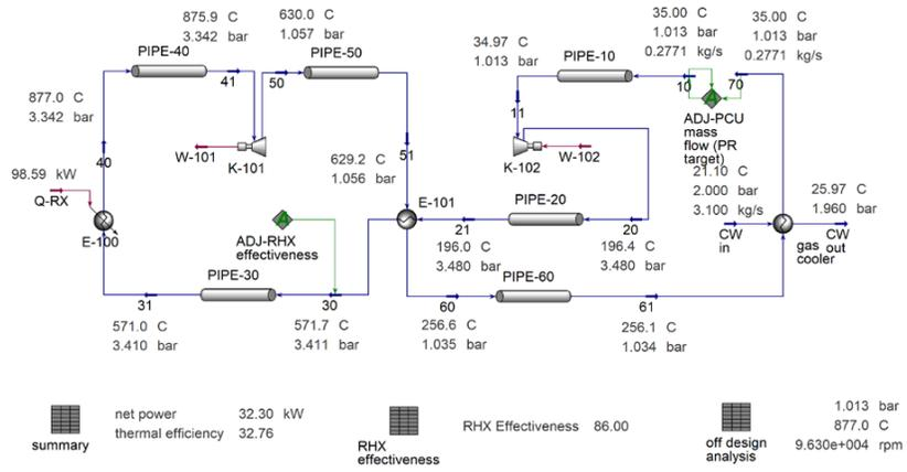
Figure 5-1. Aspen HYSYS Model Outputs for 30 kW Operation of the PCU
