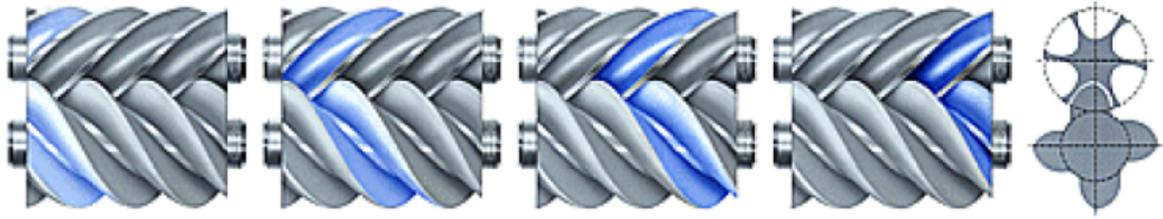
Figure 2-3. Twin-Screw Compressor General Operating Principal Diagram (Gardner Denver, n.d.)
