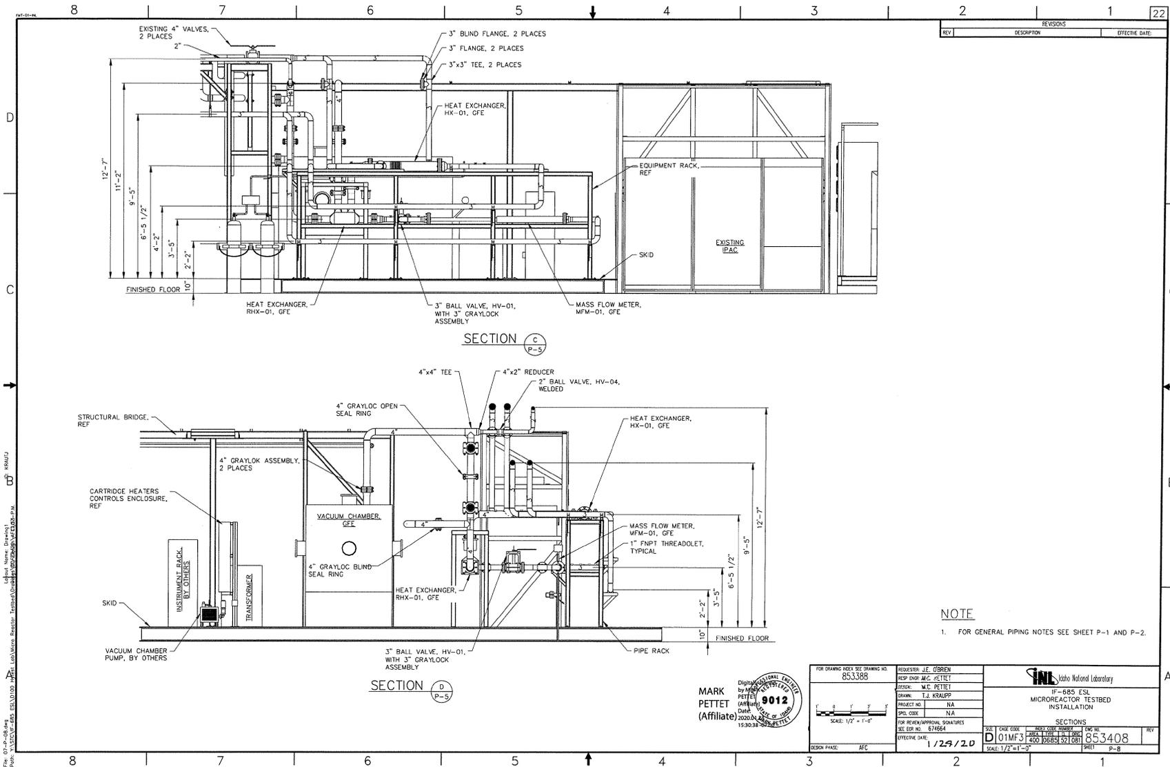
Figure A-3. Piping Construction Drawing (P-8)
