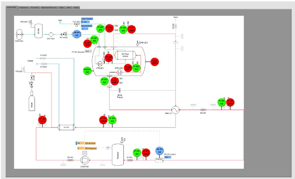
Figure 2-16. HMI for LabView VI (MAGNET Control Interface)
