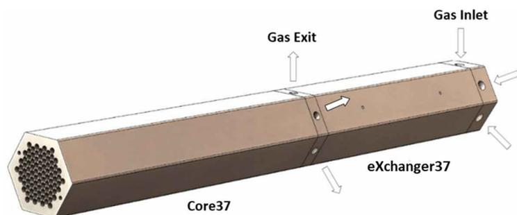
Figure 2-10. Rendering of Initial Proposed Test Article for MAGNET (Gaspar, et al., 2023)
