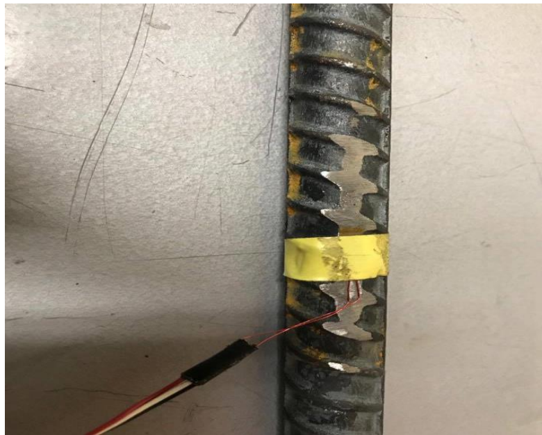
Figure 4.19: Strain gage with attached tape
