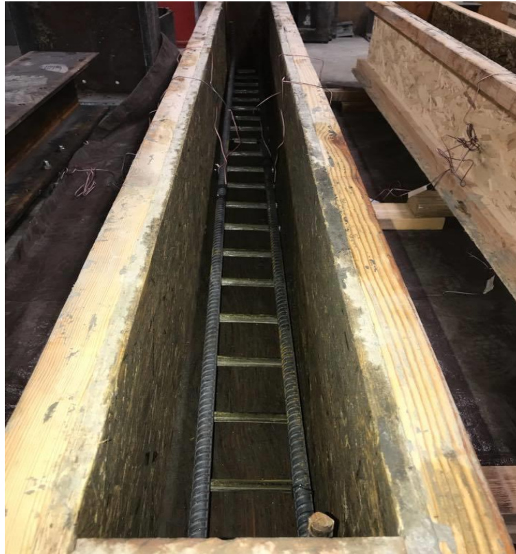
Figure 4.12: Beam Five - CFRP hybrid with steel
