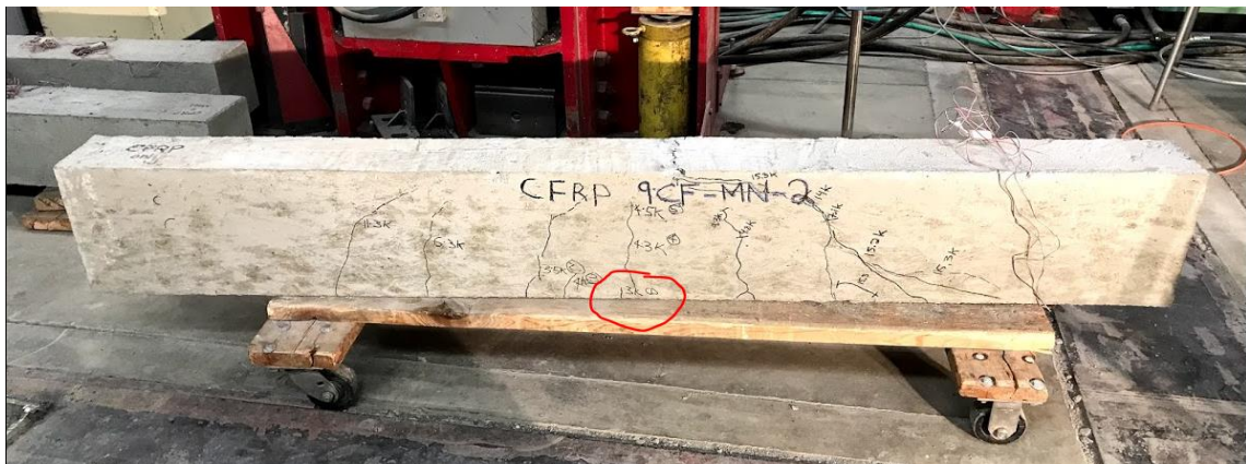
Figure 5.19: CFR- only reinforced beam after failure
