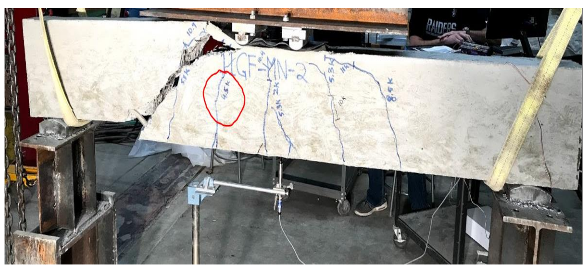
Figure 5.21: GFRP reinforce- only beam after failure
