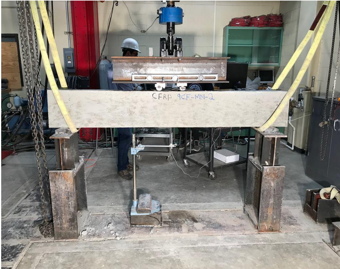
Figure 4.26: Experimental test setup of the concrete beams
