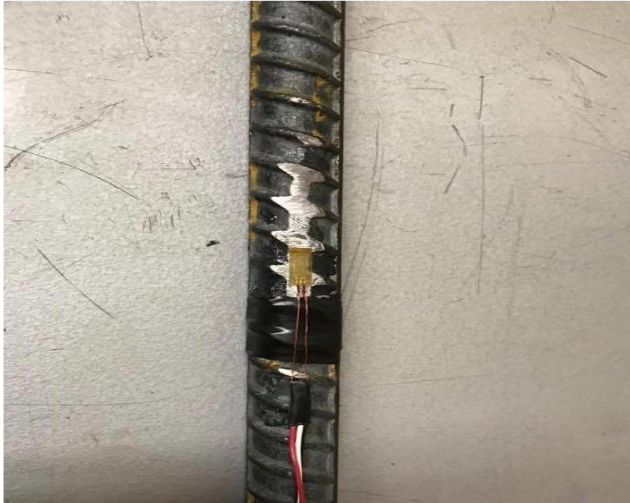
Figure 4.20: Strain gage with tape under lead wire
