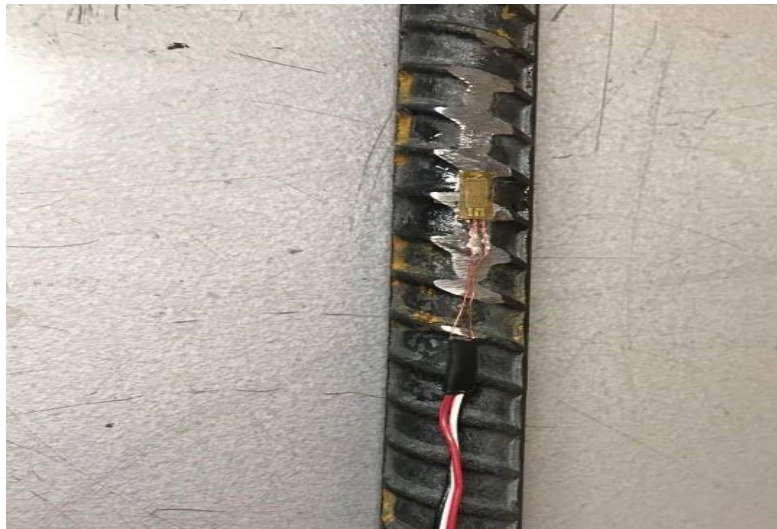
Figure 4.18: Strain gage attached to rebar with glue
