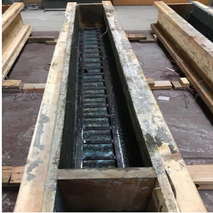
Figure 4.10: Beam Three – CFRP-only
