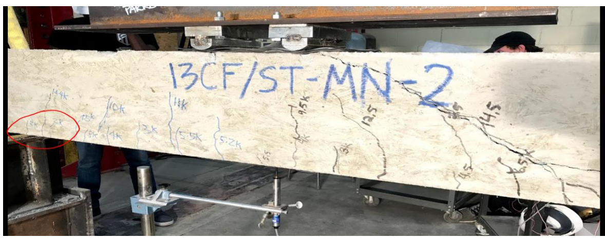
Figure 5.21: Hybrid CFRP with steel reinforced-only beam after failure
