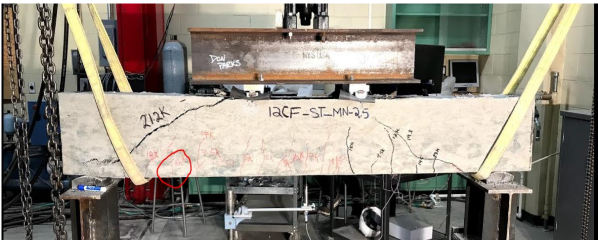
Figure 5.20: Hybrid CFRP with steel reinforced-only beam after failure
