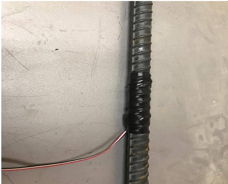
Figure 4.21: Strain gage with complete attachment
