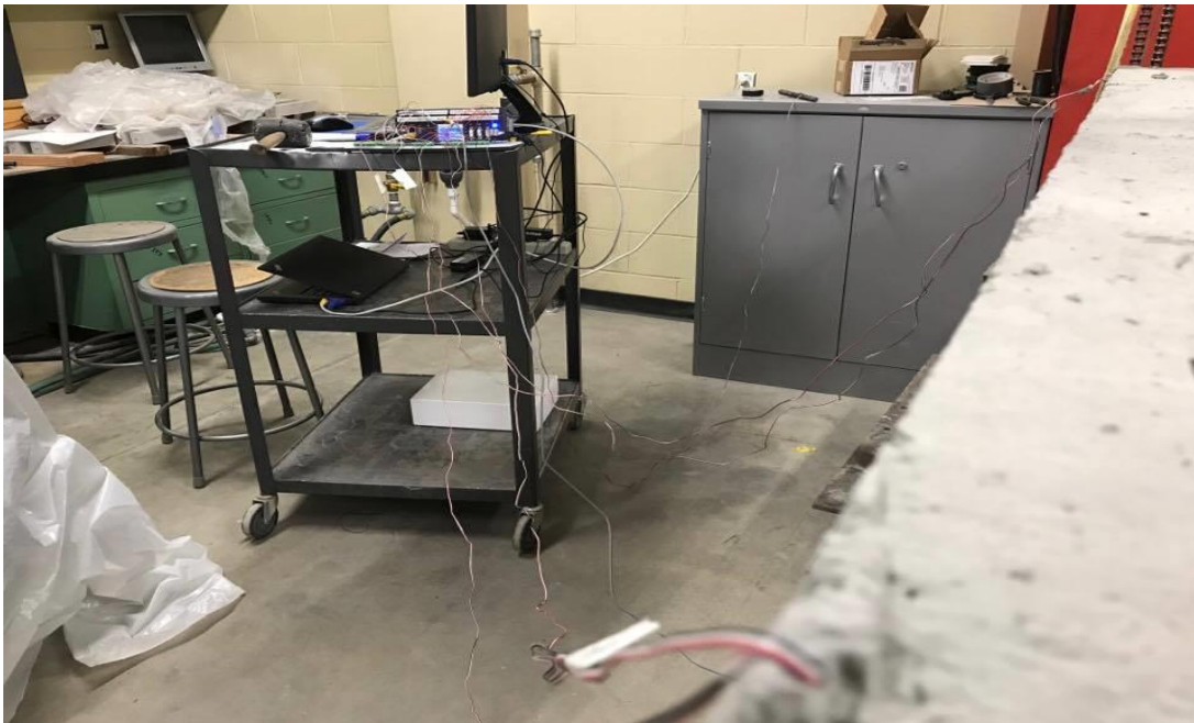
Figure 4.22: Strain gage attached to Expert Data Logger
