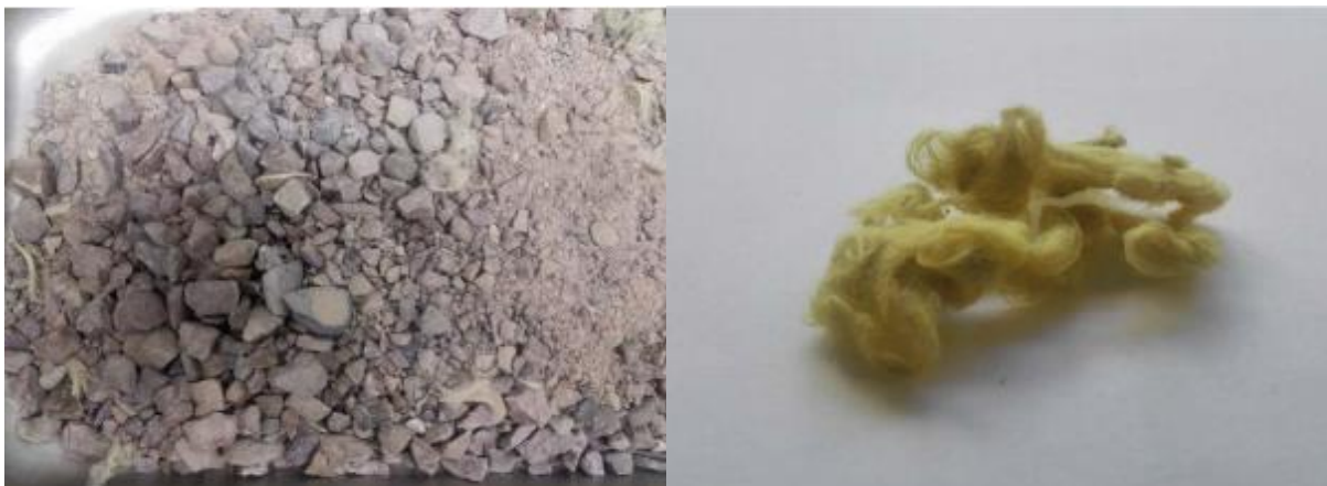
Figure 39 (a) Aggregate-Fiber Mix after Extraction (AASHTO T-164) (b) Collected Fiber #2
