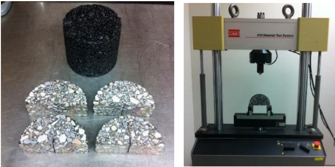
Figure 7 Fracture Test using Semicircular Notched Samples in Bending ( J_c )
