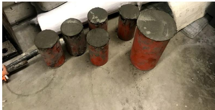
Figure 2.11. Samples for 28-day compressive strength test
