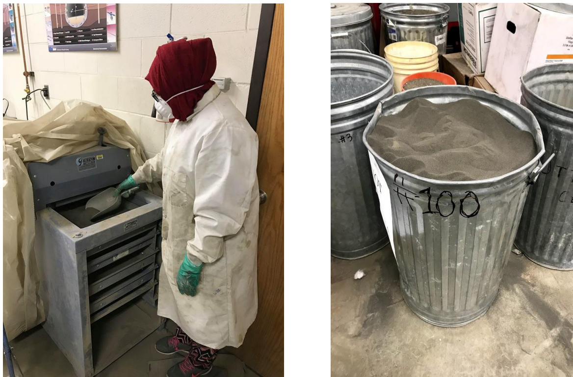
Figure 2.14 (a) Sieving procedure (b) Sieved materials (#50 passing and #100 retained)
