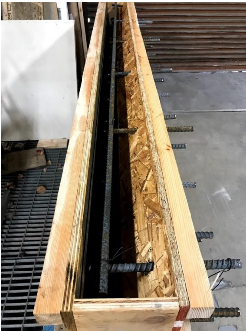
Figure 2.9. Wooden forms before pouring concrete
