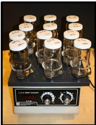
Figure 3.2 Jar Testing Set-Up
