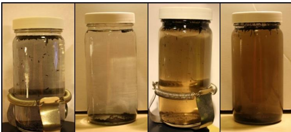
Figure 3.12 Batch Testing Observations: W biochar at 1 hour (far left) and 18 hours (2nd from left); KB biochar at 1 hour (3rd from left) and 18 hours (4th from left).
