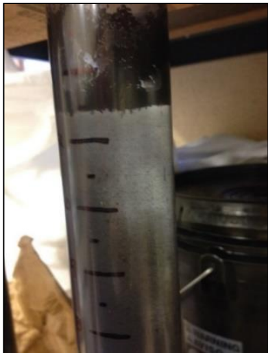
Figure 3.36. Falling Head Test: Biochar Floats
