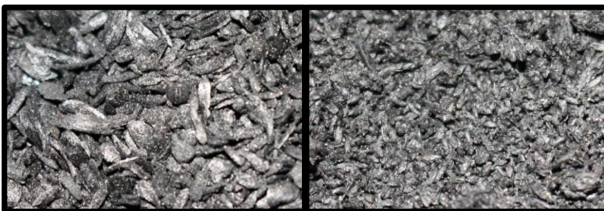
Figure 4.1 Close-up Photo of Wood (W) Biochar (left) and Kentucky Blue (KB) Grass Biochar (right)
