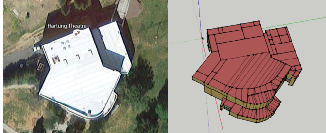
Figure 3.1: Comparison of actual (left) to modeled geometry (right). Picture of actual geometry is courtesy of Google Satellite Imagery.
