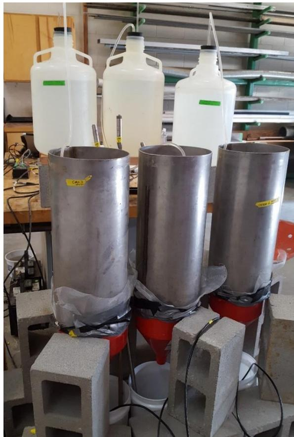
**FIGURE 1.5.** Ponded water experiment set-up with 20-gallon Mariotte bottles, pressure sensors, and EC probes in each respective drainage bucket.
