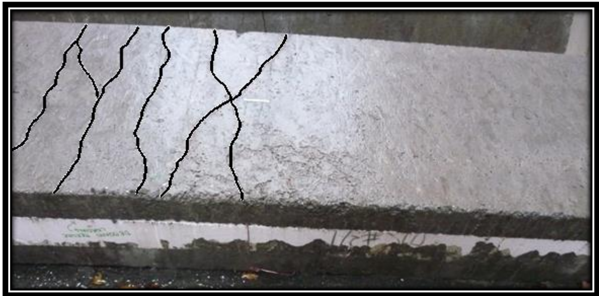
Figure 47: Segmental Connector Specimen 1—Crack Pattern (Bottom of Specimen)
