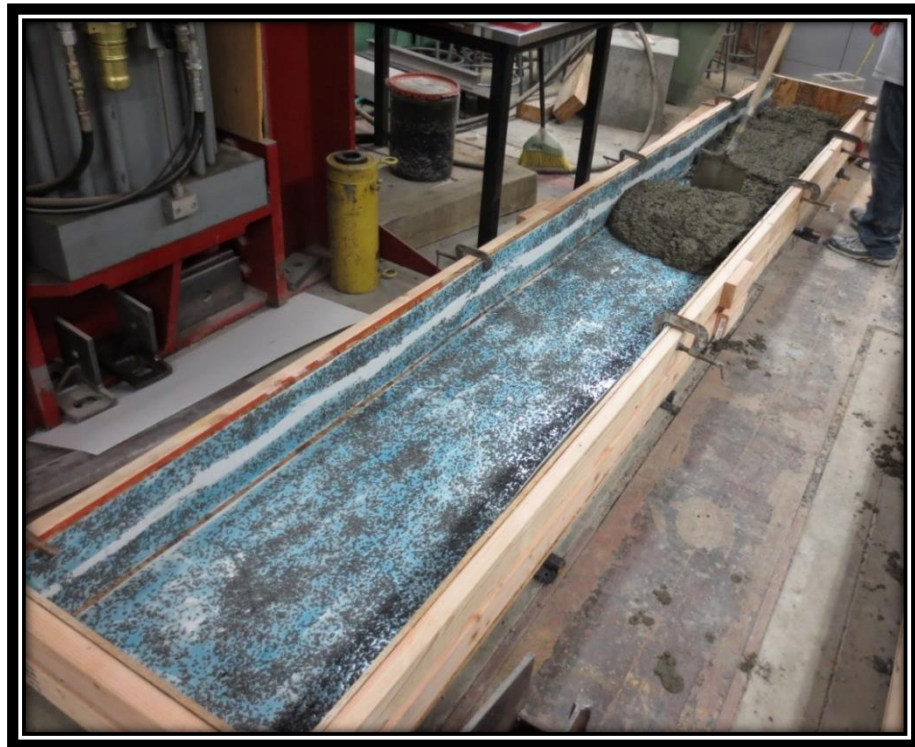
Figure 106: First Lift of Full Scale FPCS Panel
