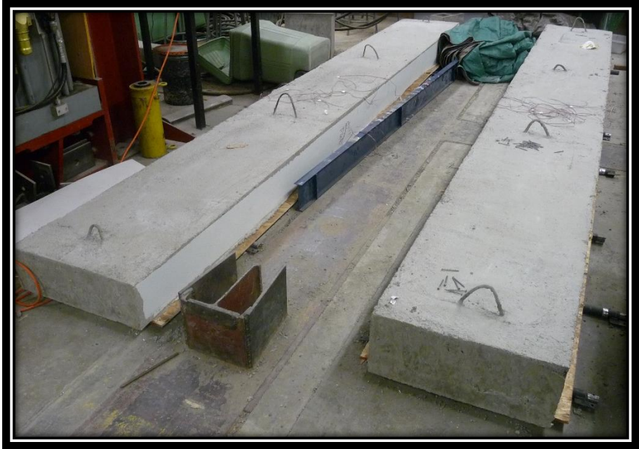
Figure 109: Cured and Stripped Full-Scale Specimens
