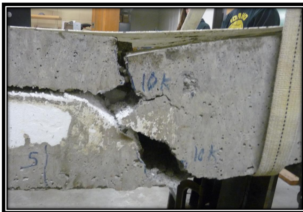
Figure 69: Shear Failure Example (Profile View)
