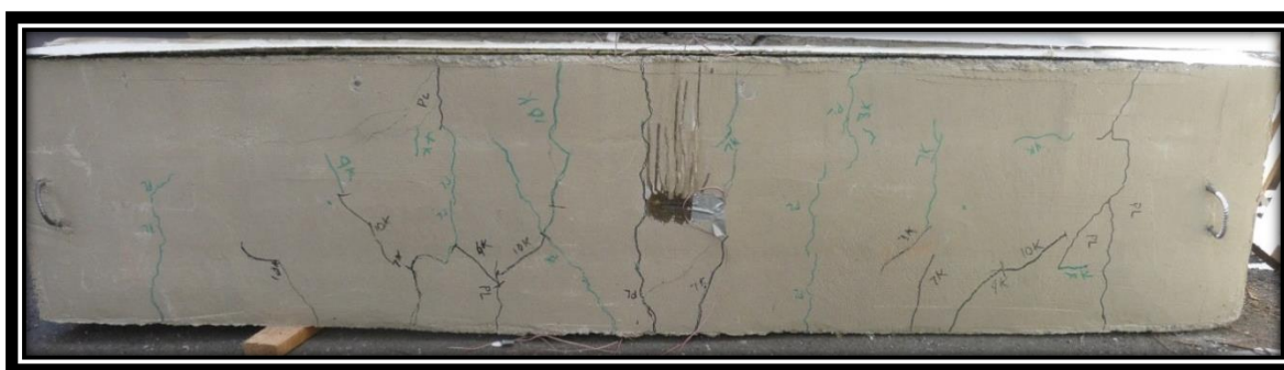
Figure 97: 10" FPCS Specimen 2—Crack Pattern (Bottom of Specimen)
