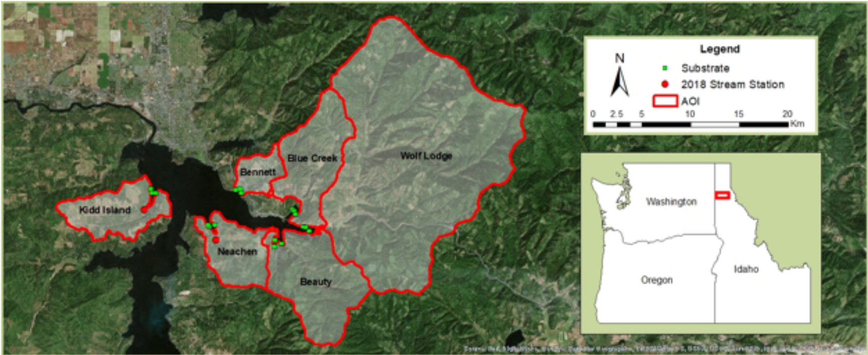
Figure 4.1: Site map of northern Coeur d'Alene Lake. Water quality and periphyton samples taken at substrate points. Area of interest (AOI) polygons represent bay watersheds generated from a 30 m DEM.
