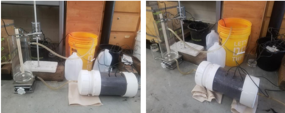
Figure 22: Completed setup of 1-dimensional soil column experiment. Sensors are inserted and float sensor maintains constant head pressure
