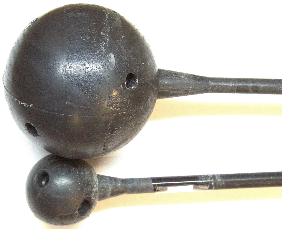
FIGURE 2.1: Ball Probe Configuration: 1.5-inch and 3-inch diameter
