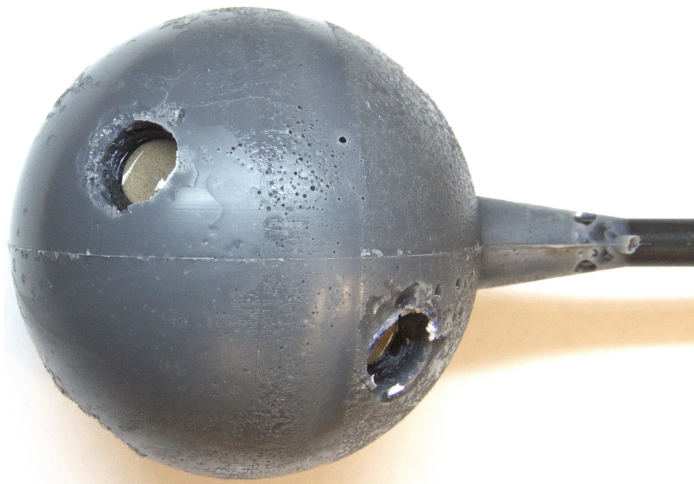
FIGURE 2.7: 3-inch Ball Probe Utilizing 12 mm Diameter Disc Electrodes
