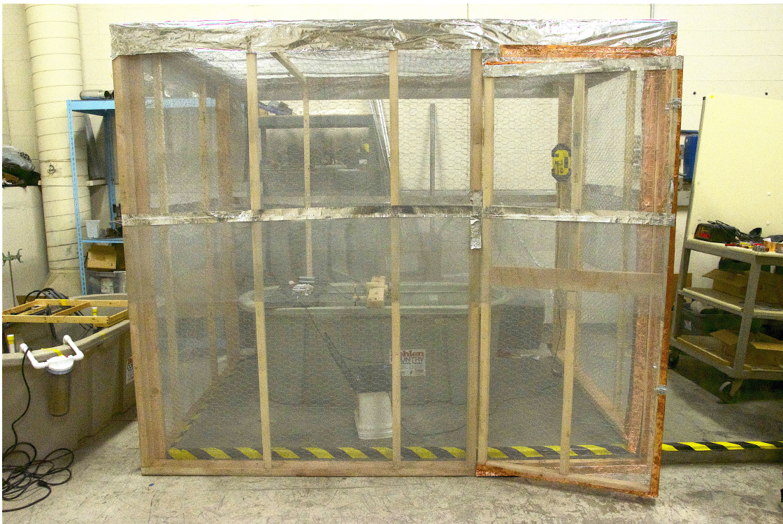
FIGURE 5.4: Faraday Cage Containing Salt Water Tank and Test Equipment
