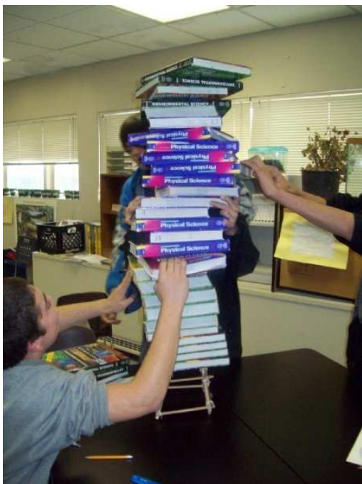
Figure 14 Students trying to collapse the Pit House model using the mass of the textbooks to apply a downward force.
