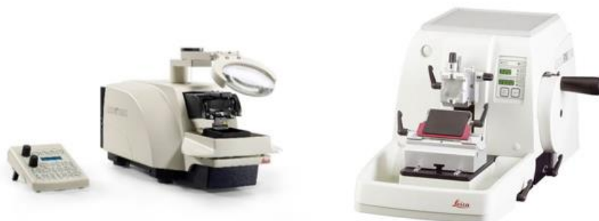
Figure 2.2: A vibratome (Leica VT 1200S) [24] (left) and a microtome (Leica RM2245) [25] (right).
