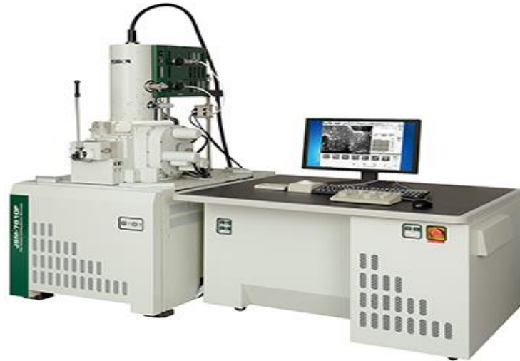
Figure 2.3: A Scanning Electron Microscope (SEM) (JEOL JSM-7610F) showing its electron beam generator column, specimen chamber, vacuum pump, monitor, and control panels [32].
