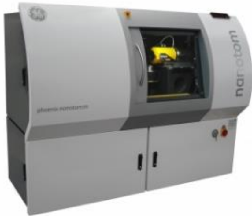
Figure 2.4: A Computed Tomography (CT) Scanner (GE Phoenix Nanotom System) showing its specimen cabinet [33].
