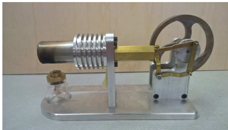
Figure 4.2: Photo of Current (2018) Design of University of Idaho Stirling Engine
