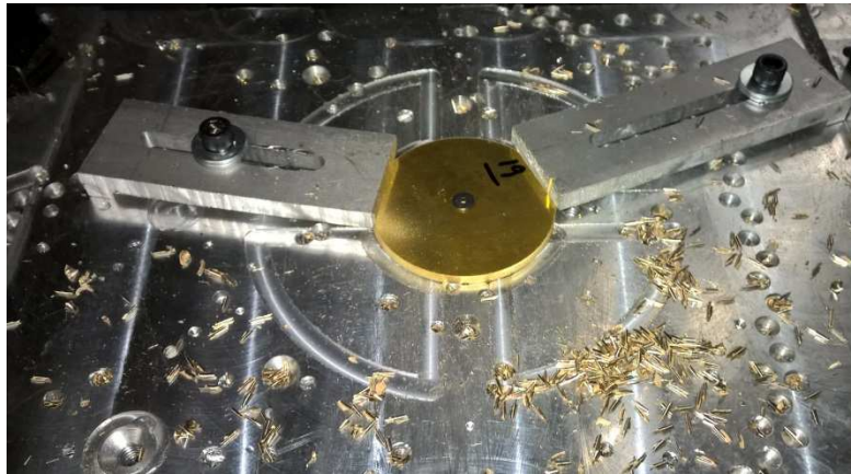
Figure 5.23: Spur Gears prior to machining
