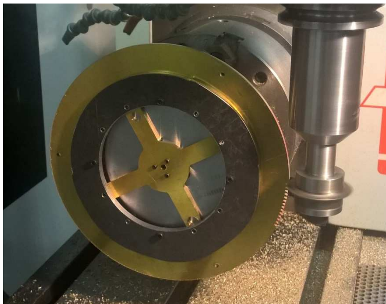
Figure 5.25: Teeth being cut into gear blank
