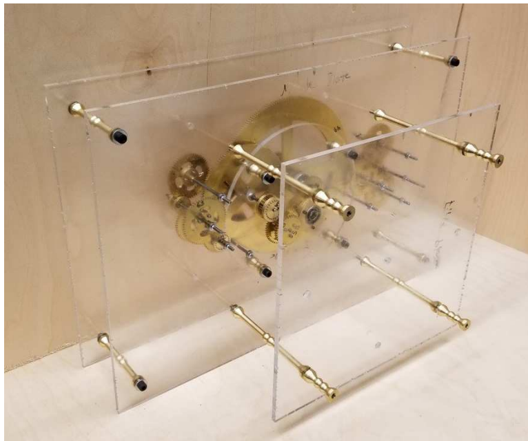
Figure 5.30: Picture third plate being installed
