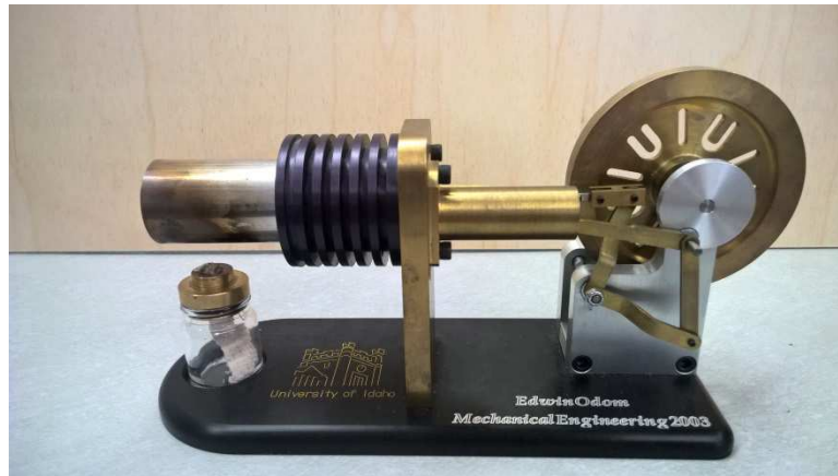
Figure 4.1: Photo of First Generation (2003) University of Idaho Stirling Engine
