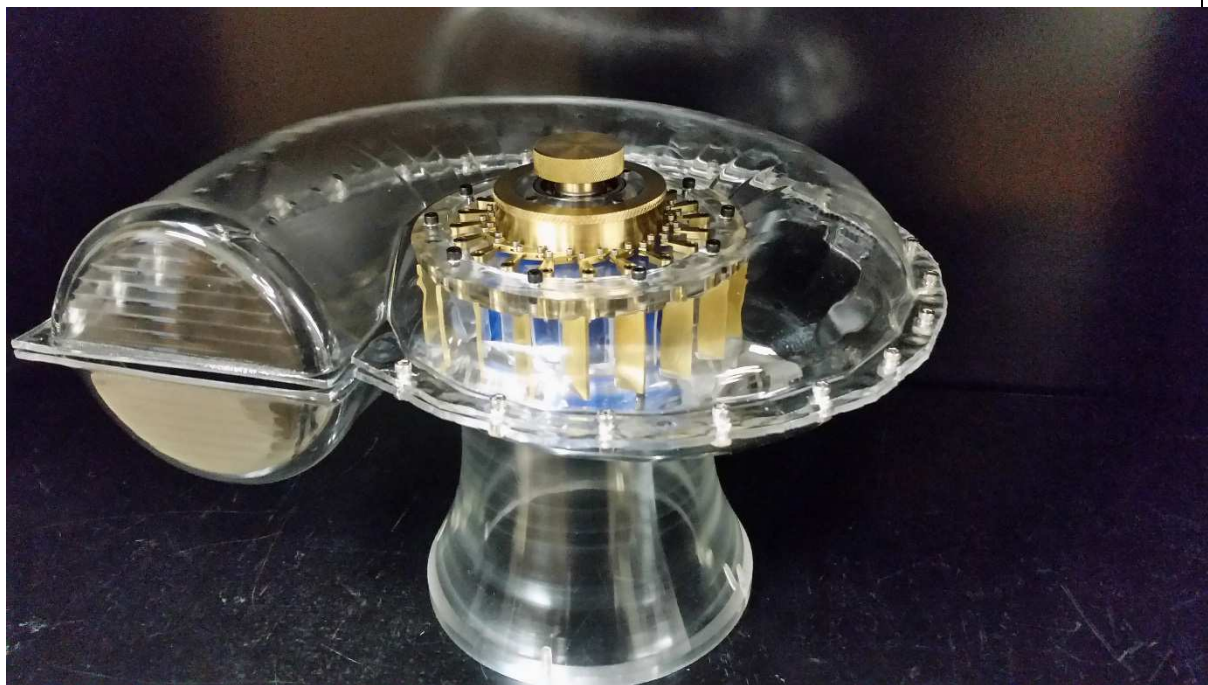
Figure 3.11: Photo of completed spiral casing on smaller (1:80) scale model
