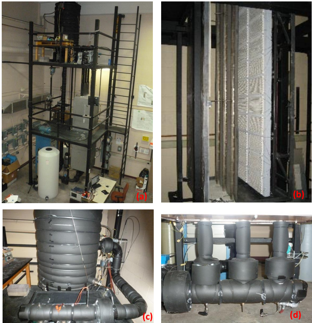
Figure 3-12: (a) Facility overview (b) Heated cavity (c) Well insulated overhead water tank and upper header (d) Lower header and three riser tubes
