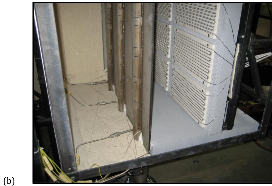
Figure 3-11: (a) Plan view of heated cavity (b) Diagram of heater, pipe and fin configuration within the heated cavity
