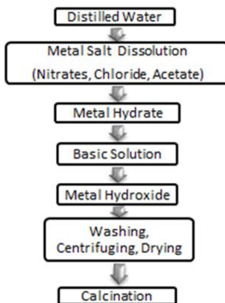
Figure 5 : Schematic of the steps in the coprecipitation synthesis technique
