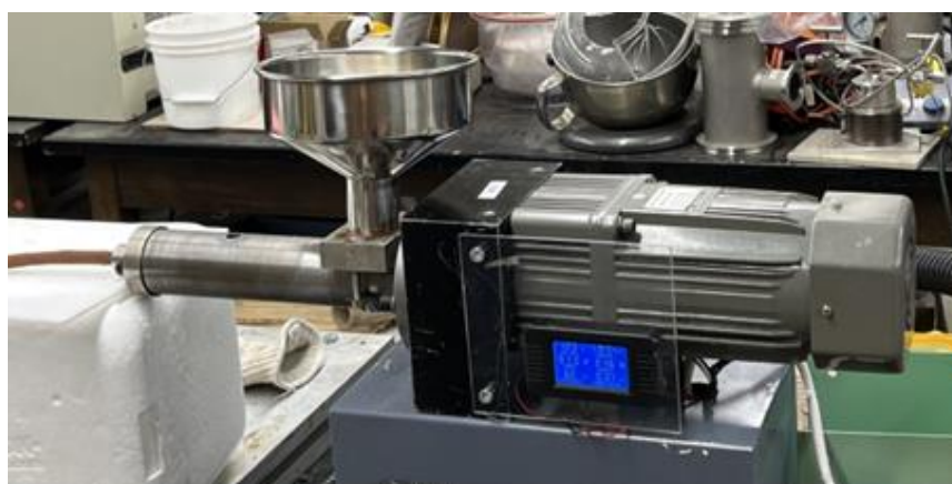
Figure A3.1: Wood-resin extruder setup
