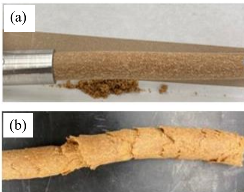
Figure 2.7: Photographs of (a) smooth extruded wood-SS (50:50) rods and (b) extruded wood-SS showing sharkskin.
