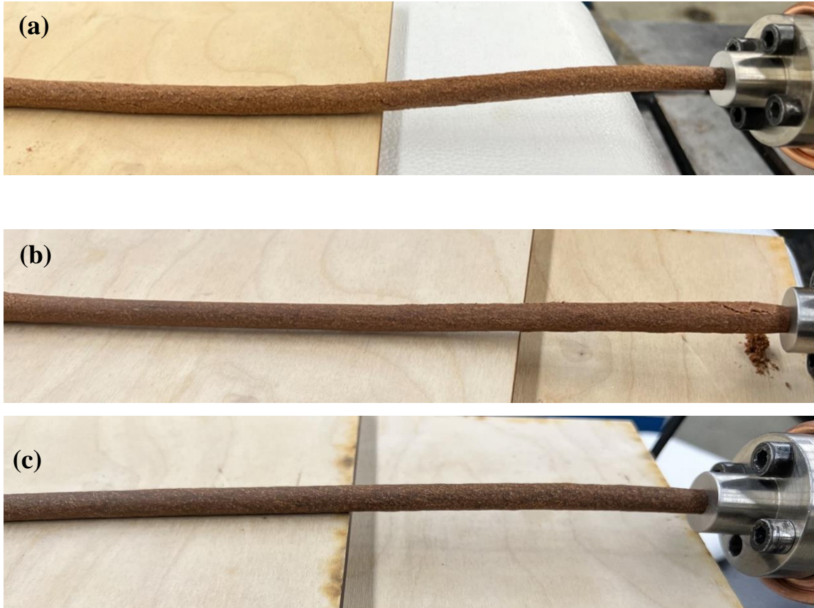
Figure 5.6: Photographs of successful extrusion runs of wood-PRF blends with the addition of modifiers showing (a) 10% SCO and (b) 10% BMES and (c) 10% GCS composites
