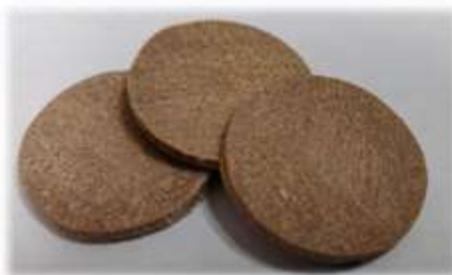
Figure 2.4: Extruded cut circular discs
