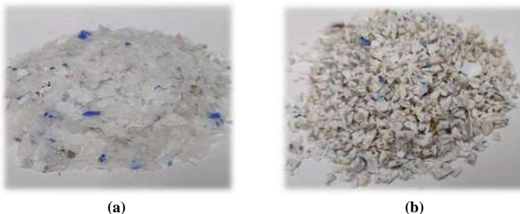
Figure 2.2: Granulated recycled polyolefins (a) HDPE and (b) PP
