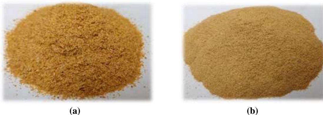
Figure 2.1: Screened rice hulls of (a)  $<1$  mm and (b)  $<0.5$  mm Particle sizes
