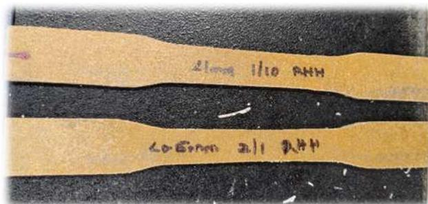
Figure 2.3: Extruded cut dog-bone samples
