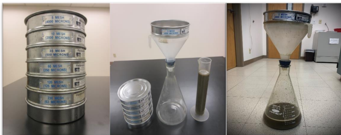
Figure 3.6: Arrangement for the wet sieving analysis.
