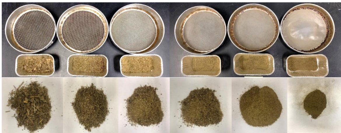
Figure 4.2: Representative sample solids retained on different sieves during the wet sieving analysis. From left to right: 4 mm, 2 mm, 0.5 mm, 0.25 mm, 0.125 mm, and 0.063 mm.
