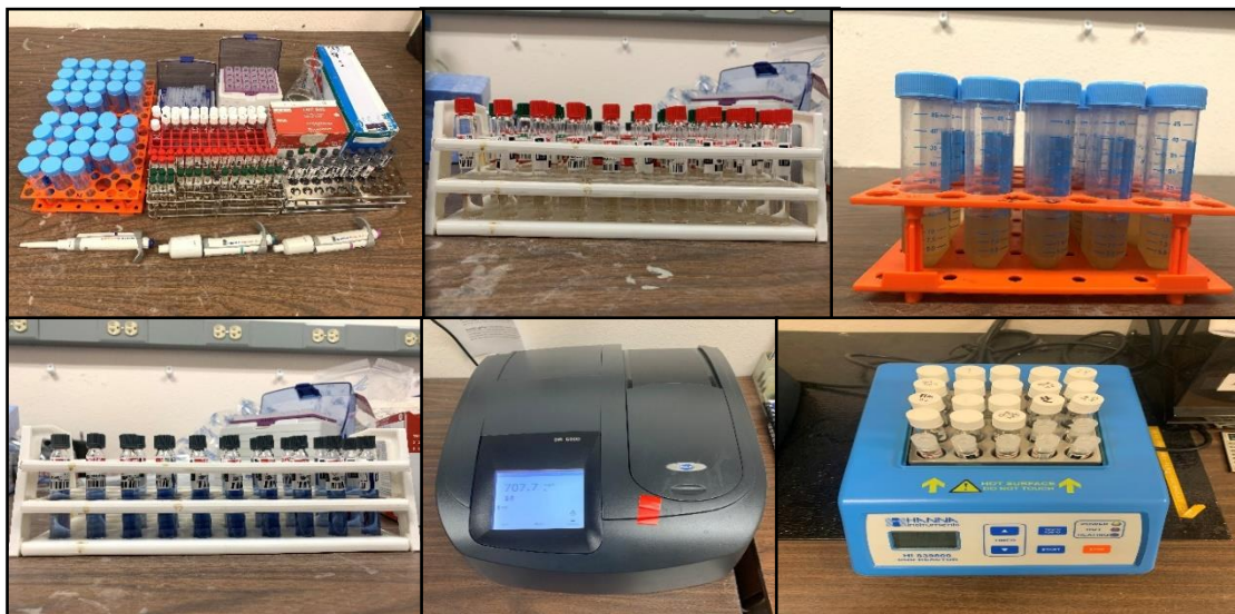
Figure 3.10: Total nitrogen and total phosphorous analysis using the Hach methods.
