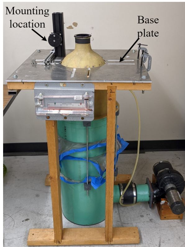
Figure 3.3: Free jet system with the surrounding base plate that will isolate the samples.
