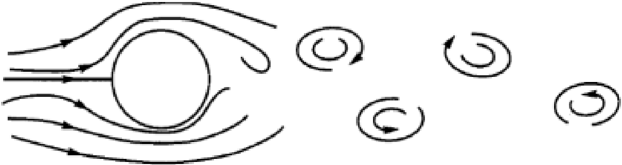
Figure 2.4: Typical vortex shedding caused by flow interference with a cylindrical bluff body. [3]
