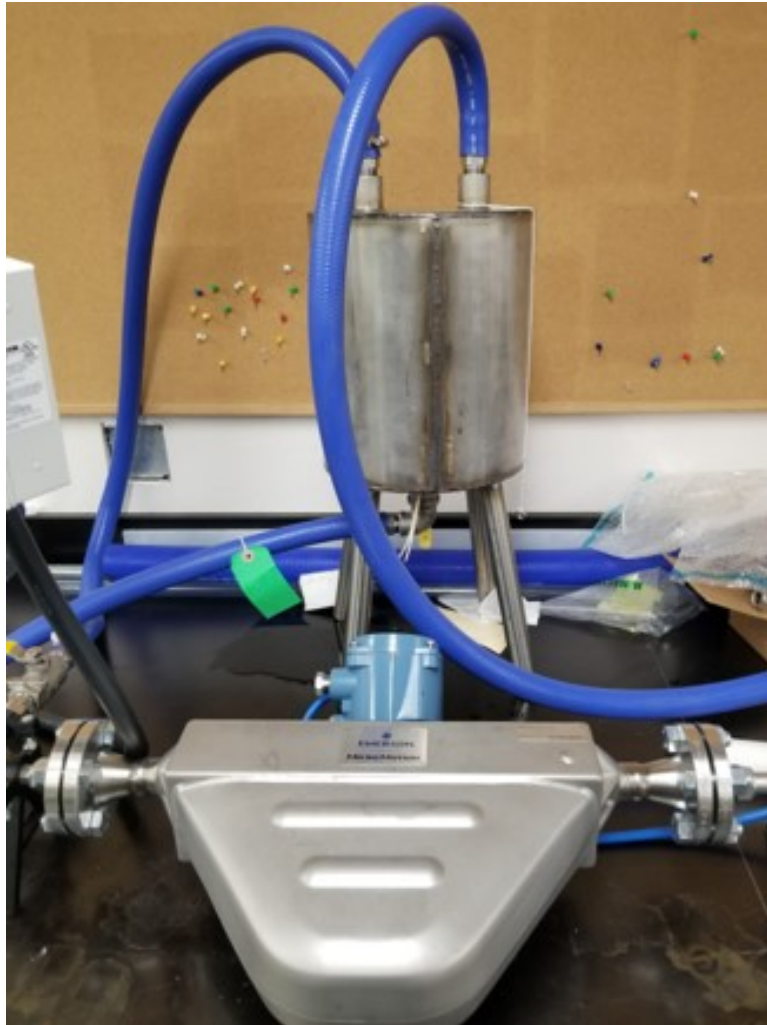
Figure 3.23: Emerson Coriolis flow meter and the tank in the back
