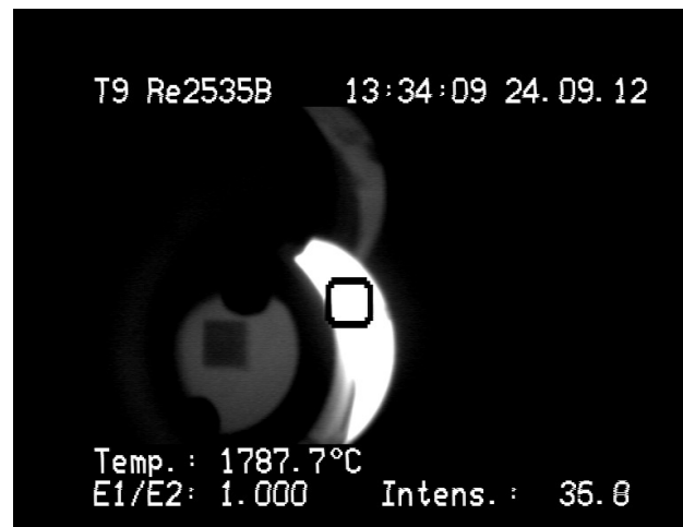
Figure 4.38. Pyrometer snapshot of sample inside crucible just before immersion.
