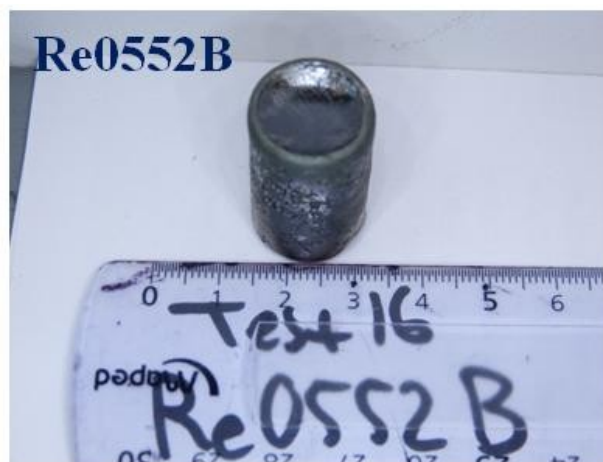
Figure 4.23. Re0552B - Test 16 (Temp. 2000°C) – SEM/EDS Results and post-test ingot.
