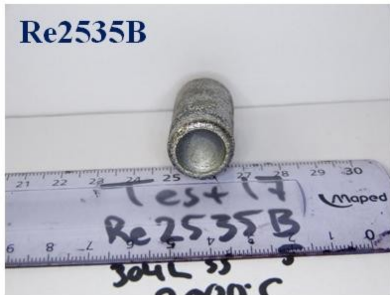
Figure 4.26. Re2535B - Test 17 (Temp. 2000°C) – Solidification curve and post-test ingot.
