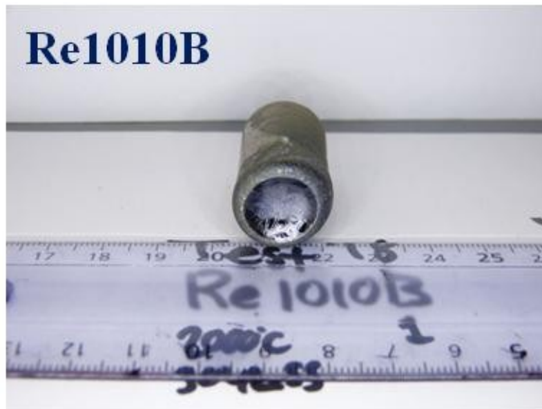
Figure 4.35. Re1010B - Test 18 (Temp. 2000°C) – Solidification curve and post-test ingot.
