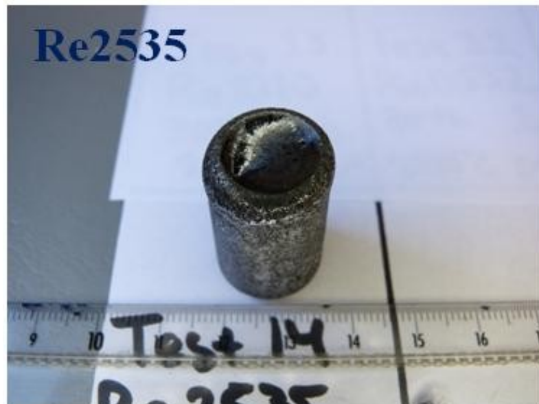
Figure 4.24. Re2535 - Test 14 (Temp. 2000°C) – Solidification curve and post-test ingot.
