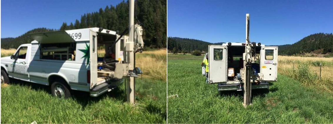
Figure 10: The Geoprobe coring device used to extract sediment cores from the floodplain.
