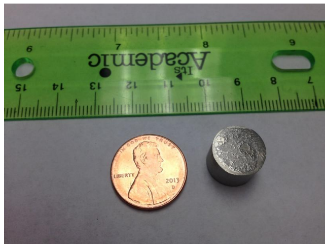
Figure 8.1. A macroscopic view of the SPSed Ni–20Cr–1.2Y 2 O 3 specimen (sample mass – 10 g)
