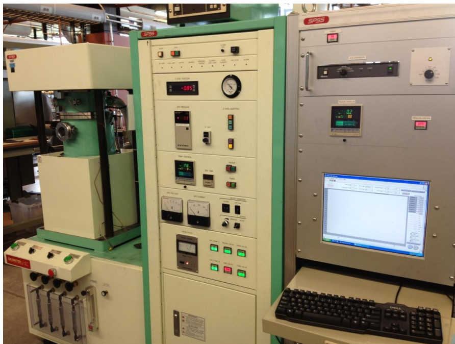
Figure 1.17. A Dr. Sinter SPS-515S unit including sintering chamber, electrical unit and monitor / control unit from left to right
