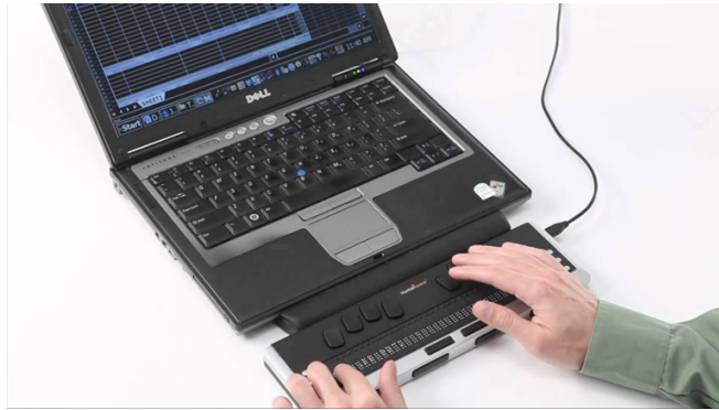
Figure 1.1 Image of the HumanWare Braille display connected to a laptop computer. Note the eight buttons located directly above the braille strip used for typing and navigation.
