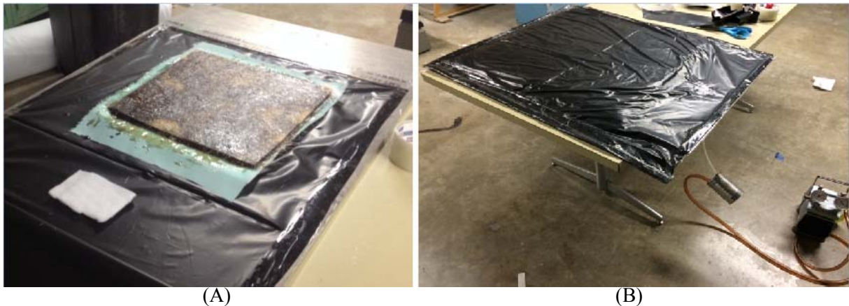
Figure 23: Vacuum Bagging Process A) FRP sealing bag B) After sealing bag
