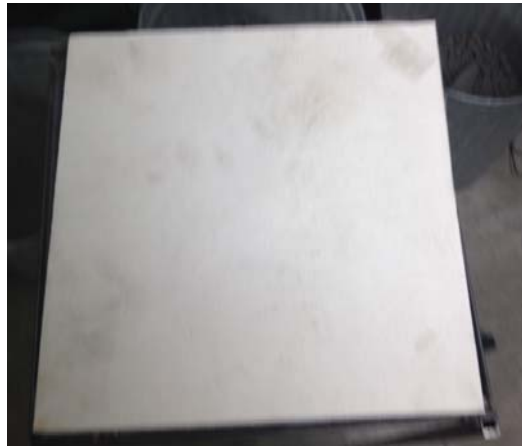
Figure 12: Top of Gypsum after Double Panel Test
