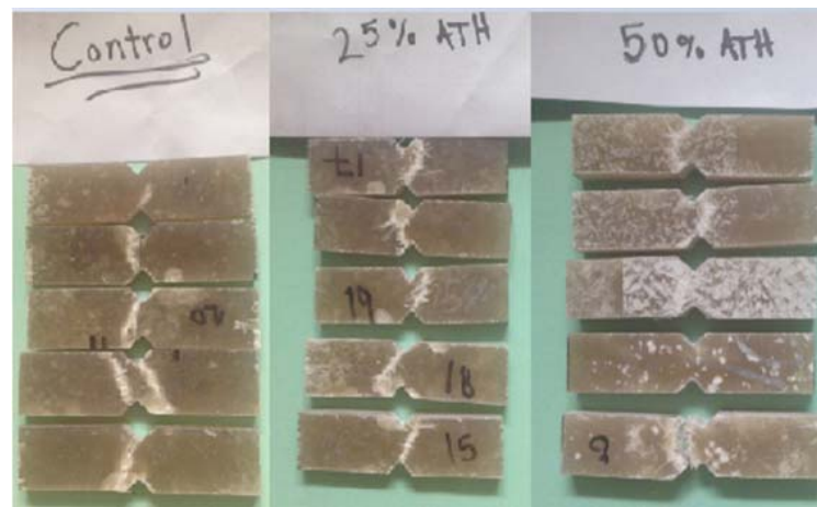
Figure 51: Failure Mode for (A) Control, (B) 25% ATH, (C) 50% ATH
