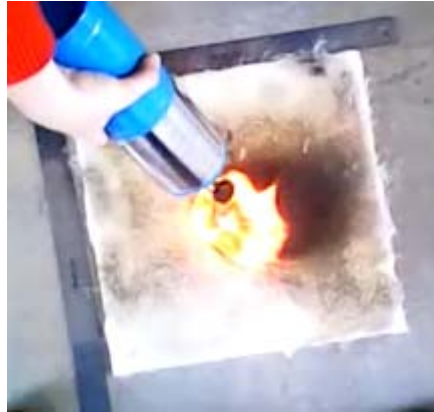
Figure 14: Flame Spread Test Setup
