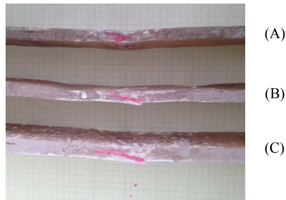
Figure 48: Failure Mode, Side View of (A) Control, (B) 25% ATH, (C) 50% ATH 5.3.3 Shear (ASTM C 1292)
