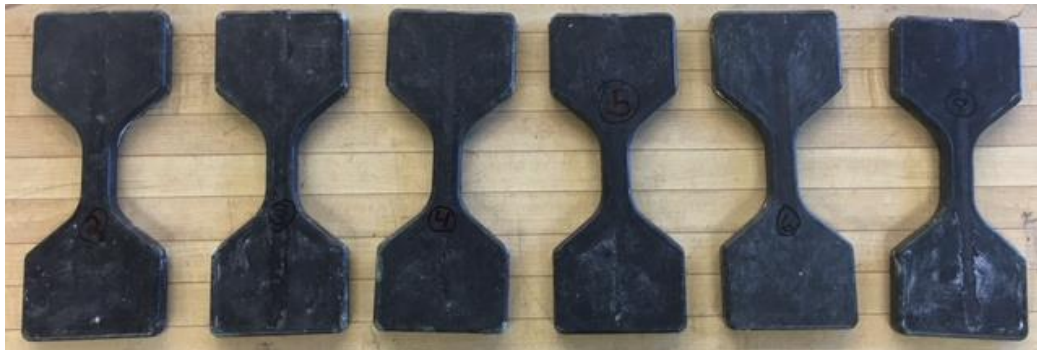
Figure 26: Specimens after curing
