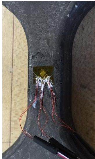
Figure 29: Installed stacked rosette strain gage
