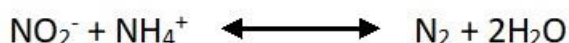
Figure 1.2. Transformation of nitrite to nitrogen gas by the enzymes nitrite reductase, hydrazine synthase, and hydrazine dehydrogenase.
