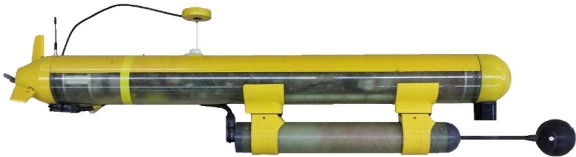
**Figure 2.1:** UI AUV Equipped with electric field probe and additional sensor array.
