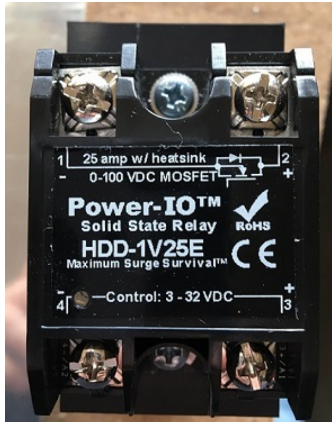
Figure 3.11: Power ID MOSFET relay
