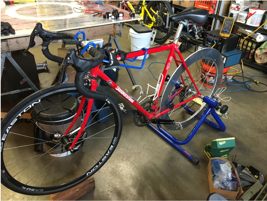
Figure 4.2: Set-up of the Computer Controlled Eddy Current Brake Bicycle Trainer.
