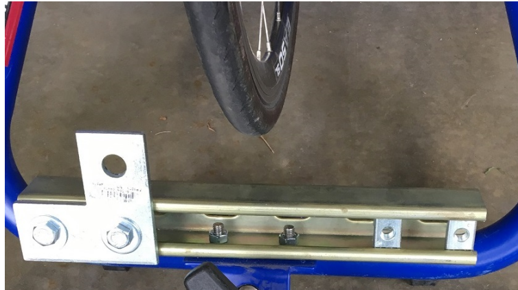
Figure 3.4: Unistrut mounted to the trainer
