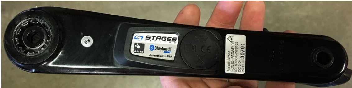
Figure 3.16: Bicycle crank with Stages Cycling power meter attached
