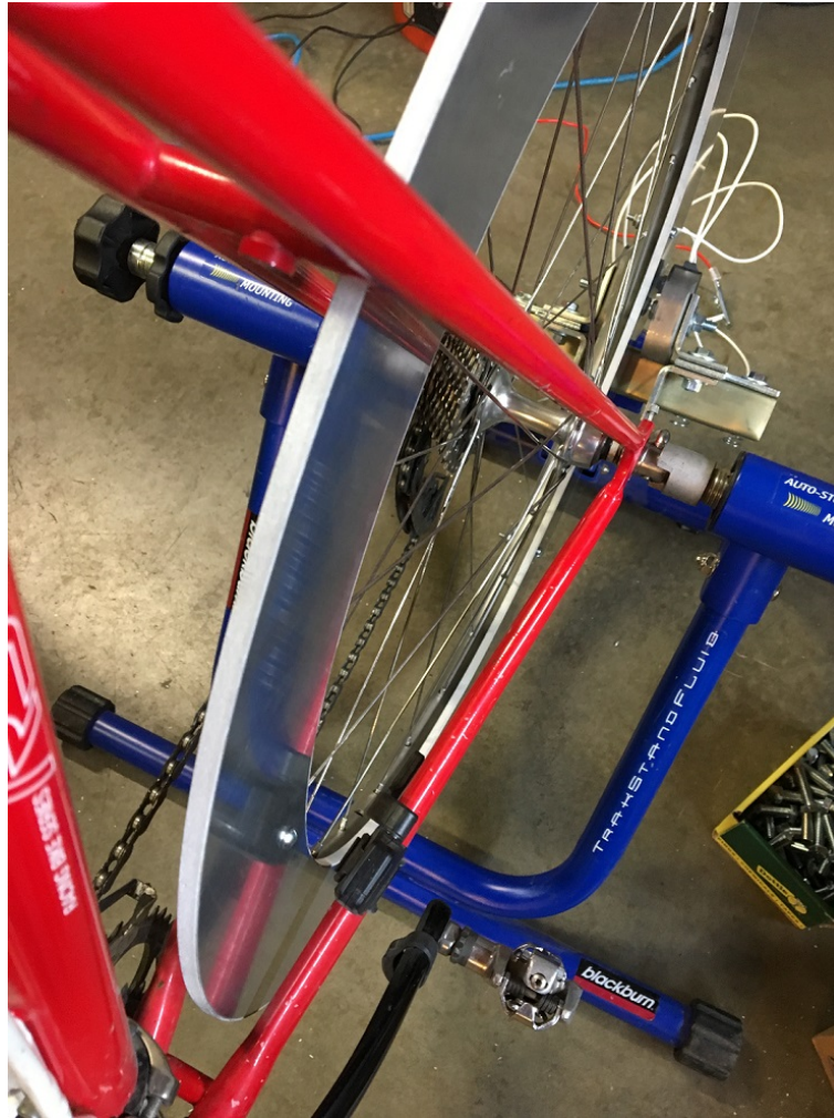
Figure 3.7: Aluminum donut mounted to rear wheel
