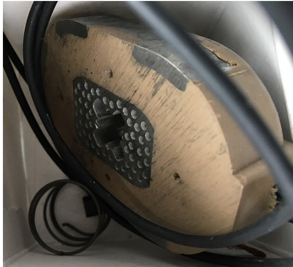
Figure 3.8: Automobile industry trailer brake electromagnets used in the eddy current brake
